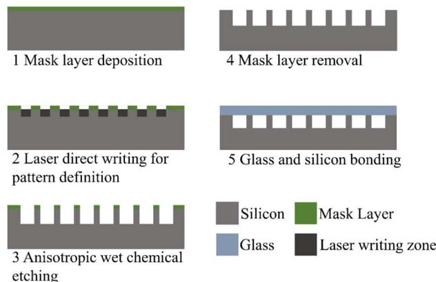
Fig. 1 Fabrication process of silicon-based qPCR chips. Including deposition of the  $\text{SiN}_x$  protective layer, laser direct writing to define the microchannel pattern, wet chemical etching to form the microchannel, removal of  $\text{SiN}_x$ , and silicon-glass bonding.
