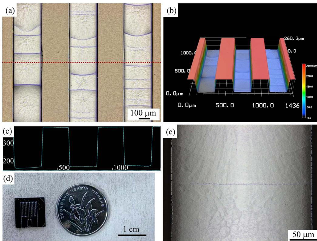
Fig. 4 (a) Microscopic image of microchannels on chips. The position of the red dotted line in the image corresponds to the section outline in (c). (b) 3D image of microchannels created by laser (658 nm) scanning. (c) The profile curve of the microchannel cross-section. (d) A photo of a chip compared to a coin in size. (e) High-magnification microscopic images of the bottom of microchannels.
