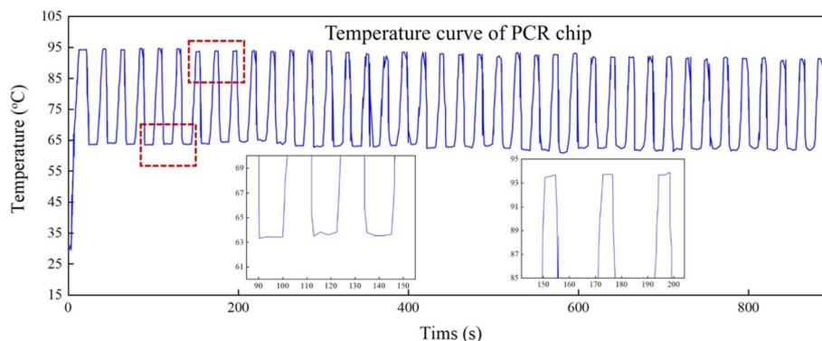
Fig. 5 Thermal cycling curve of on-chip qPCR.
