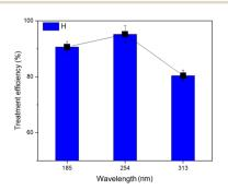
Fig. 4 Effect of the light wavelength on the efficiency of TNT treatment (pH 3,  $C_{\text{H}_2\text{O}_2} = 40$  mM,  $C_{\text{Fe}^0} = 2$  mM, T = 40 °C, CTNTO = 50 mg L<sup>-1</sup>, ultrasound = 40 kHz and 60 W, reaction time = 30 min).
