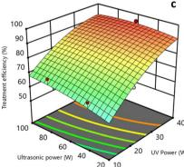
Fig. 8 Impact of ultrasonic power (a) and light power (b) and their combination (c) (pH 3,  $C_{\rm H_2O_2}=40$  mM,  $C_{\rm Fe^0}=2$  mM,  $C_{\rm TNT}^0=50$  mg L $^{-1}$ , ultrasound = 40 kHz, UV = 254 nm, reaction time = 20 min).
