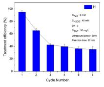
Fig. 10 TNT treatment efficiency of the reused nZVI catalyst in the sono-photo-Fenton-like process (pH 3,  $C_{H_2O_2} = 40$  mM,  $C_{Fe^0} = 2$  mM,  $C_{\text{TNT}}^0 = 50 \text{ mg L}^{-1}$ , ultrasonic = 40 kHz and 60 W, UV = 254 nm and 10 W, reaction time = 30 min)
