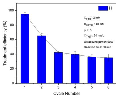
Fig. 10 TNT treatment efficiency of the reused nZVI catalyst in the sono-photo-Fenton-like process (pH 3,  $C_{\text{H}_2\text{O}_2} = 40$  mM,  $C_{\text{Fe}^0} = 2$  mM,  $C_{\text{TNT}}^0 = 50$  mg L<sup>-1</sup>, ultrasonic = 40 kHz and 60 W, UV = 254 nm and 10 W, reaction time = 30 min).
