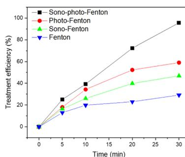
Fig. 9 Comparison of the efficiency of TNT treatment among various advanced oxidation methods (pH 3,  $C_{H_2O_2} = 40$  mM,  $C_{Fe^0} = 2$  mM,  $C_{TNT}^0 = 50$  mg L<sup>-1</sup>, reaction time = 30 min).
