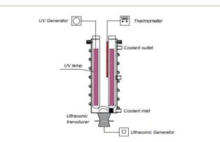
Fig. 11 Design of the experimental reactor for the sono-photo-Fenton process.
