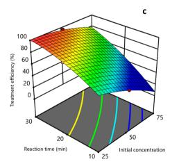
Fig. 7 Effect of the initial TNT concentration (a), reaction time (b), and their combination (c) on TNT treatment efficiency (pH 3,  $C_{H_2O_2}$  = 40 mM,  $C_{\text{Fe}^0} = 2$  mM, ultrasound = 40 kHz and 60 W, UV = 254 nm and 10 W).
