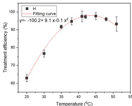
Fig. 2 Effect of temperature on TNT treatment efficiency in aqueous solution with pH 3,  $C_{H_2O_2} = 40$  mM,  $C_{Fe^0} = 2$  mM,  $C_{TNT}^0 = 50$  mg L<sup>-1</sup>, ultrasound = 40 kHz and 60 W, UV = 254 nm and 10 W, reaction time 30 min.
