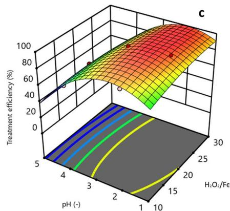
Fig. 6 Effect of the H<sub>2</sub>O<sub>2</sub>/Fe<sup>0</sup> ratio (a), pH (b) and their combination (c) on the efficiency of TNT treatment ( $C_{\text{Fe}^0} = 2$  mM,  $C_{\text{TNT}}^0 = 50$  mg L<sup>-1</sup>, ultrasound = 40 kHz and 60 W, UV = 254 nm and 10 W, reaction time = 30 min).
