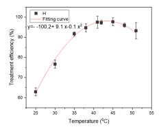
Fig. 2 Effect of temperature on TNT treatment efficiency in aqueous solution with pH 3,  $C_{\rm H_2O_2}=40$  mM,  $C_{\rm Fe^0}=2$  mM,  $C_{\rm TNT}^0=50$  mg L $^{-1}$ , ultrasound = 40 kHz and 60 W, UV = 254 nm and 10 W, reaction time 30 min.
