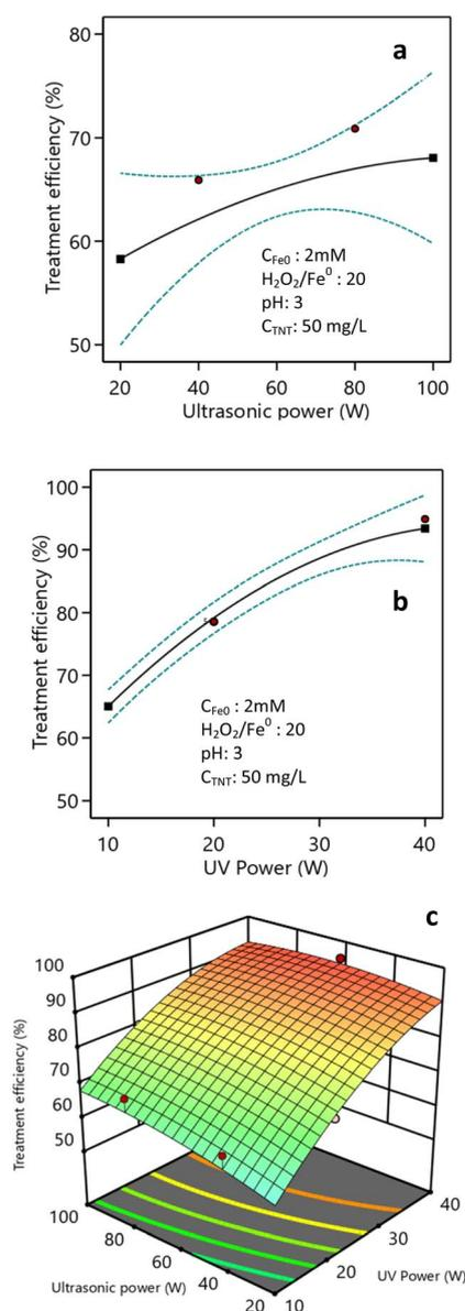
Fig. 8 Impact of ultrasonic power (a) and light power (b) and their combination (c) (pH 3,  $C_{H_2O_2} = 40$  mM,  $C_{Fe^0} = 2$  mM,  $C_{TNT}^0 = 50$  mg L<sup>-1</sup>, ultrasound = 40 kHz, UV = 254 nm, reaction time = 20 min).
