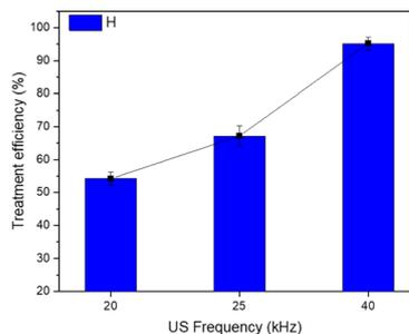
Fig. 5 Effect of ultrasound frequency on the efficiency of TNT treatment. (pH 3,  $C_{\text{H}_2\text{O}_2} = 40$  mM,  $C_{\text{Fe}^0} = 2$  mM,  $T = 40$  °C,  $C_{\text{TNT}0} = 50$  mg L<sup>-1</sup>, UV = 254 nm and 10 W, reaction time = 30 min).
