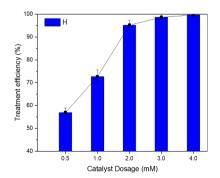
Fig. 3 Impact of the dosage of zero-valent iron nanoparticles (nZVI) catalyst on the efficiency of TNT treatment (pH 3,  $C_{\rm H_2O_2}=40$  mM, T=40 °C,  $C_{\rm TNT}^0=50$  mg L $^{-1}$ , ultrasound = 40 kHz and 60 W, UV = 254 nm and 10 W, reaction time = 30 min).
