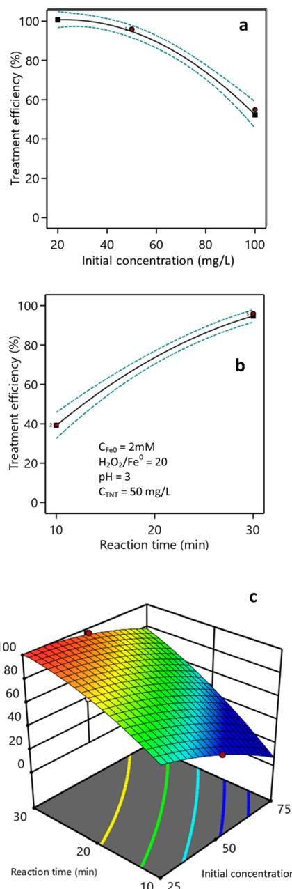
Fig. 7 Effect of the initial TNT concentration (a), reaction time (b), and their combination (c) on TNT treatment efficiency (pH 3, C<sub>H<sub>2</sub>O<sub>2</sub></sub> = 40 mM, C<sub>Fe<sup>0</sup></sub> = 2 mM, ultrasound = 40 kHz and 60 W, UV = 254 nm and 10 W).
