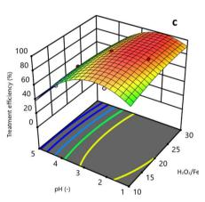
Fig. 6 Effect of the  $\rm H_2O_2/Fe^0$  ratio (a), pH (b) and their combination (c) on the efficiency of TNT treatment ( $C_{\rm Fe^0} = 2$  mM,  $C_{\rm TNT}^0 = 50$  mg L $^{-1}$ , ultrasound = 40 kHz and 60 W, UV = 254 nm and 10 W, reaction time = 30 min).
