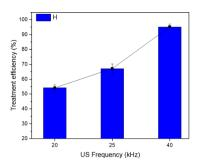
Fig. 5 Effect of ultrasound frequency on the efficiency of TNT treatment. (pH 3,  $C_{\rm H_2O_2}=40$  mM,  $C_{\rm Fe^0}=2$  mM, T=40 °C, CTNT0 = 50 mg L<sup>-1</sup>, UV = 254 nm and 10 W, reaction time = 30 min).
