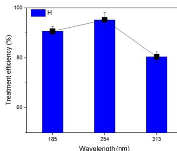
Fig. 4 Effect of the light wavelength on the efficiency of TNT treatment (pH 3,  $C_{H_2O_2} = 40$  mM,  $C_{Fe^0} = 2$  mM,  $T = 40$  °C,  $C_{TNT}^0 = 50$  mg L<sup>-1</sup>, ultrasound = 40 kHz and 60 W, reaction time = 30 min).
