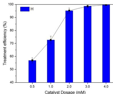
Fig. 3 Impact of the dosage of zero-valent iron nanoparticles (nZVI) catalyst on the efficiency of TNT treatment (pH 3,  $C_{H_2O_2} = 40$  mM,  $T = 40$  °C,  $C_{TNT}^0 = 50$  mg L<sup>-1</sup>, ultrasound = 40 kHz and 60 W, UV = 254 nm and 10 W, reaction time = 30 min).
