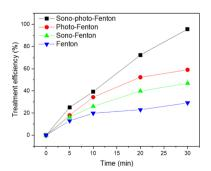
Fig. 9 Comparison of the efficiency of TNT treatment among various advanced oxidation methods (pH 3,  $C_{\rm H_2O_2}=40$  mM,  $C_{\rm Fe^0}=2$  mM,  $C_{\rm TNT}^0=50$  mg L $^{-1}$ , reaction time = 30 min).
