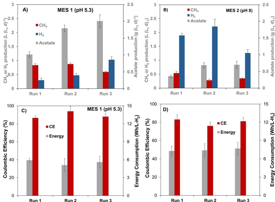
Fig. 2 Comparison of acetate, CH<sub>4</sub> and H<sub>2</sub> production in (A) MES-1 and (B) MES-2 inoculated with bioaugmented mixed microbial populations in Run #2 and Run #3 and with non-bioaugmented mixed populations in Run #1 and the corresponding coulombic efficiencies and energy consumption in (C) MES-1 and (D) MES-2 respectively.
