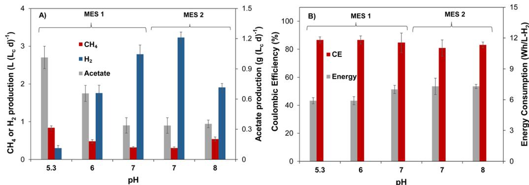
Fig. 1 (A) Steady-state values of (A) acetate, CH<sub>4</sub> and H<sub>2</sub> production observed at different levels of cathodic pH in MES cells inoculated with mixed microbial population of anaerobic sludge (Run #1); and (B) coulombic efficiency and energy consumption. MES-1 was operated at low to moderate pH levels and MES-2 operated at moderate to high pH levels.
