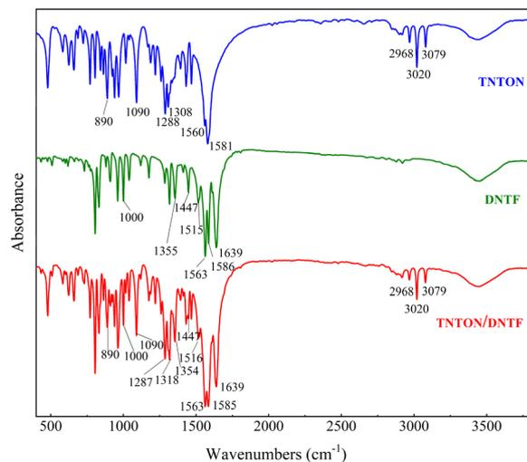
Fig. 7 IR spectra of TNTON, DNTF and the TNTON/DNTF eutectic.
