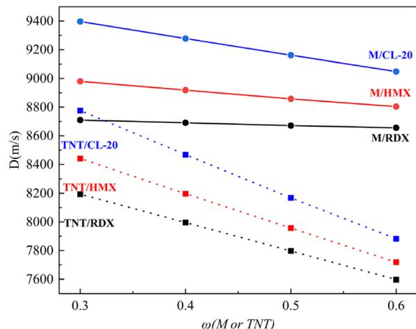
Fig. 12 Detonation velocity of TNTON/DNTF eutectic base (TNT) fused cast explosives.
