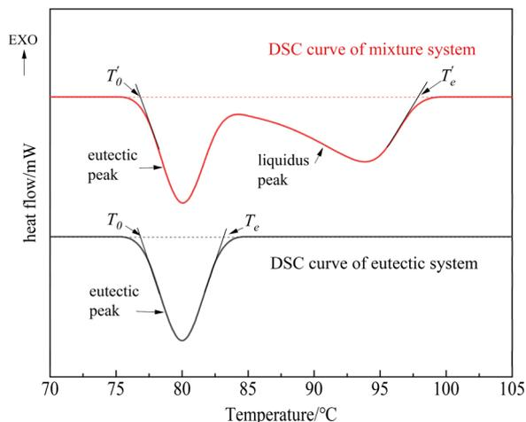
Fig. 5 Schematic diagram of liquefaction temperature obtained from DSC curves of the binary system.<sup>16,24,25</sup>
