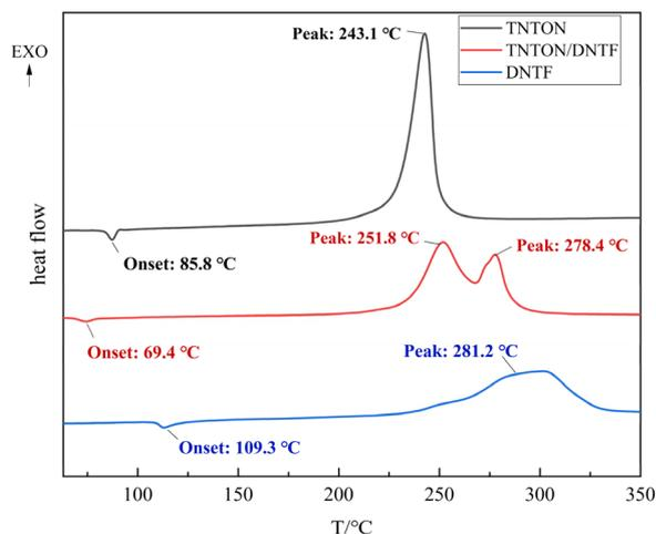
Fig. 3 DSC curves of TNTON and DNTF.
