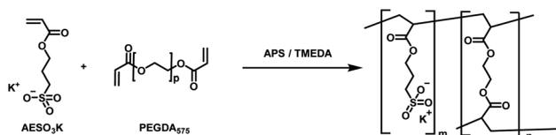
Fig. 1 Synthesis of AESO<sub>3</sub>-PEGDA<sub>575</sub>-hydrogels with APS and TMEDA initiator system for radical polymerization.
