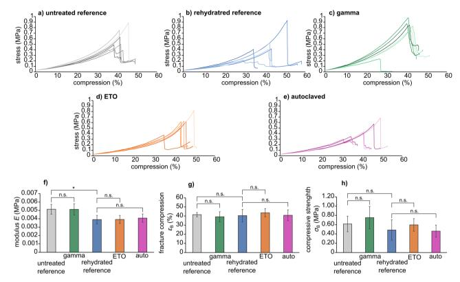
Fig. 3 Compression curves of AESO<sub>3</sub>-PEGDA<sub>575</sub>-hydrogels without and after sterilization as function of stress [MPa] *versus* compression [%] (a– e) and bar graphs of average values of modulus E (f), fracture compression  $\varepsilon_B$  (g) and compressive strength  $\sigma_B$  (h). Asterisks indicate significance (P < 0.05), n.s. indicate no significance (P < 0.05) as determined by two-tailed t test.
