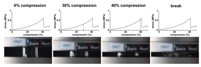
Fig. 4 Exemplary images of the compression behaviour of pAESO<sub>3</sub>-PEGDA<sub>575</sub> hydrogel reference at 0%, 30%, 40% compression and at compression at break (42%). The dashed lines show the respective compression (%) for the corresponding video capture frame.
