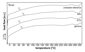
Fig. 7 Exemplary heating curves of pAESO<sub>3</sub>-PEGDA<sub>575</sub> hydrogel without and after sterilization. Position of glass transition ( $T_q$ ) is indicated.
