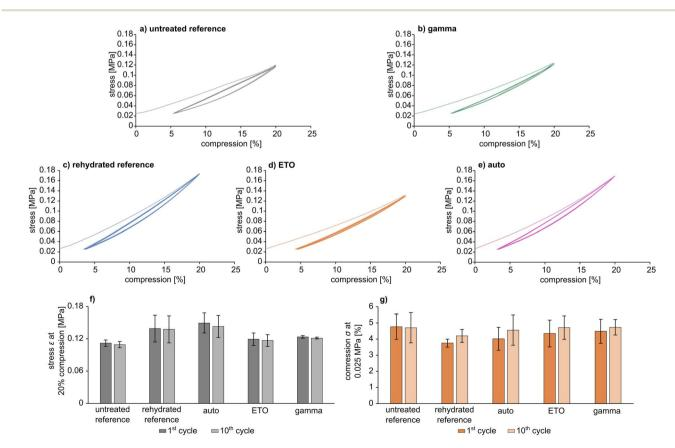
Fig. 5 Exemplary cyclic compression curves for pAESO<sub>3</sub> hydrogel (a and c) and pAESO<sub>3</sub> hydrogel after sterilization (b, d and e) and characteristic parameters stress  $\varepsilon$  at 20% compression (f) and compression  $\sigma$  at 0.025 MPa (g) calculated as mean value for n=3.
