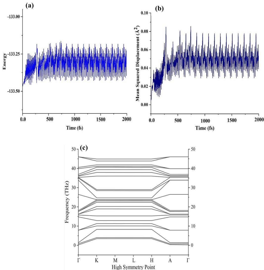
Fig. 4 AIMD analysis and phonon dispersion spectrum of BCN; (a) energy vs. time, (b) MSD vs. time, and (c) phonon dispersion spectrum.
