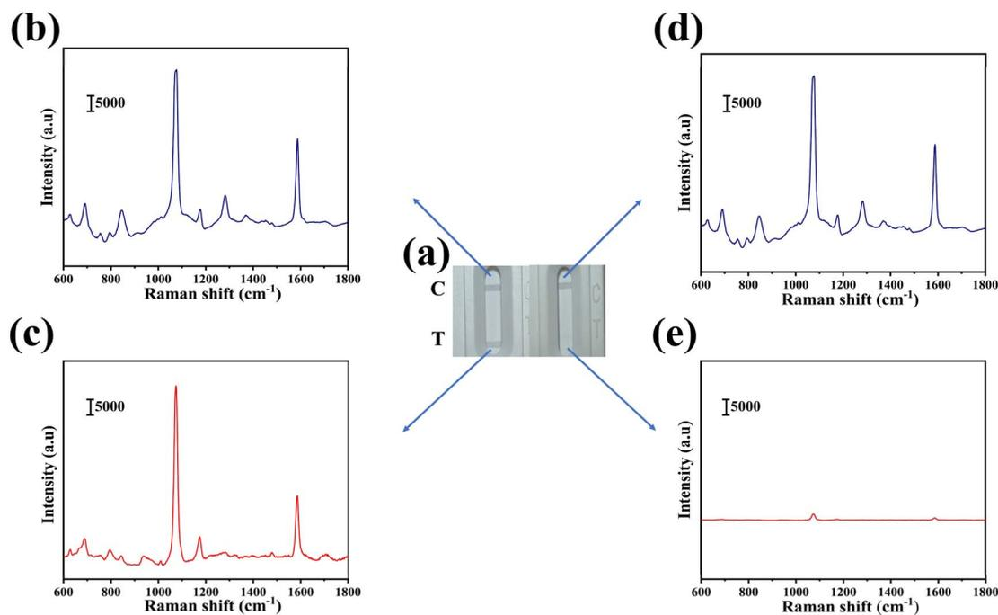
Fig. 3 (a) Color rendering results of strips at two different concentrations ( $0 \mu\text{g mL}^{-1}$  and  $1000 \mu\text{g mL}^{-1}$  miR-96-5p), when the concentration of miR-96-5p was  $0 \mu\text{g mL}^{-1}$ , (b) the SERS spectra on the C line and (c) SERS spectrum on the T line of the strips were obtained, when the concentration of miR-96-5p was  $1000 \mu\text{g mL}^{-1}$ , (d) SERS spectra on the C line and (e) SERS spectrum on the T line of the strips were obtained.
