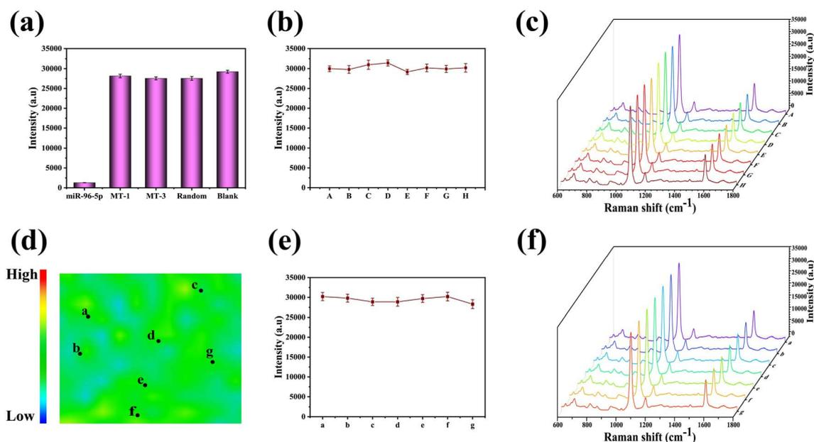
Fig. 5 (a) SERS intensities of different miRNAs at  $1073 \text{ cm}^{-1}$  at the same concentration, (b) the SERS intensity and (c) spectrum of the T line when measured with different batches of SERS-LFA strips, (d) 4-MBA SERS mapping on the SERS-LFA strips T line, when seven points 'a-g' were arbitrarily selected on the T line, (e) the SERS intensity and (f) SERS spectrum of 4-MBA at the characteristic peak of  $1073 \text{ cm}^{-1}$  were randomly selected.
