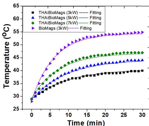
Fig. 4 Induction heating curve of magnetic Mn–Zn nanoferrite  $(\text{Mn, Zn})\text{Fe}_2\text{O}_4$  particles, BioMags and THAiBioMags with Box-Lucas (eqn (2)) fitting operating at 3, 5 and 7 kW with a frequency of 130 kHz.
