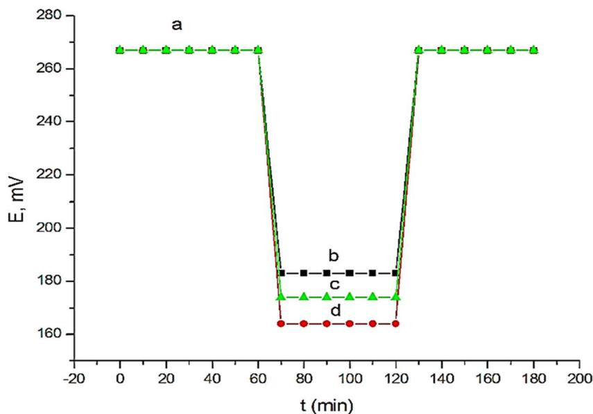
Fig. 5 Water layer test for the proposed sensor. Measurements were recorded in  $1.0 \times 10^{-3} \text{ mol L}^{-1}$  Prx<sup>+</sup> (a) and  $1.0 \times 10^{-3} \text{ mol L}^{-1}$  fluoxetine hydrochloride (b) or nisoxetine hydrochloride (c) or dapoxetine hydrochloride (d).
