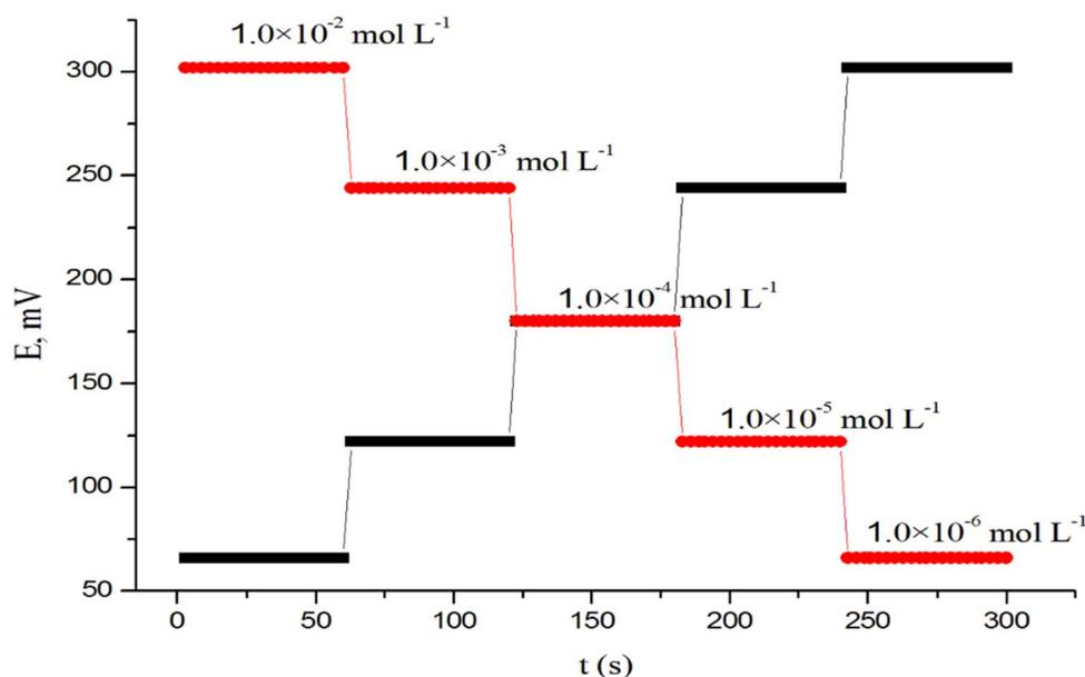
Fig. 3 Dynamic response time of CPS for step changes in the concentrations of Prx<sup>+</sup> from low to high and vice versa.
