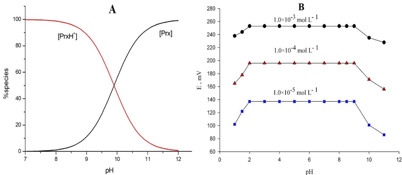
Fig. 4 (A) Representative concentration distribution diagram for Prx<sup>+</sup> species, (B) effect of the pH of test solutions on the potential response of CPS.
