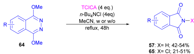
Scheme 43 Synthesis of phthalimides from 1,4-dimethoxyphthalazines.
