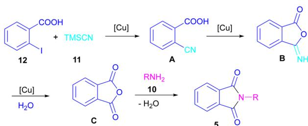
Scheme 7 Proposed mechanism for Cu-cyanation-annulation-aminolysis reaction toward phthalimides.
