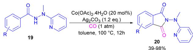
Scheme 10 Co-catalyzed carbonylation of benzoyl hydrazide derivatives.
