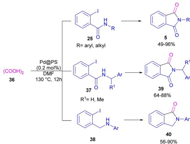
Scheme 24 Pd@PS-catalyzed reactions of 2-iodobenzamides and 2-iodobenzylanilines with oxalic acid.
