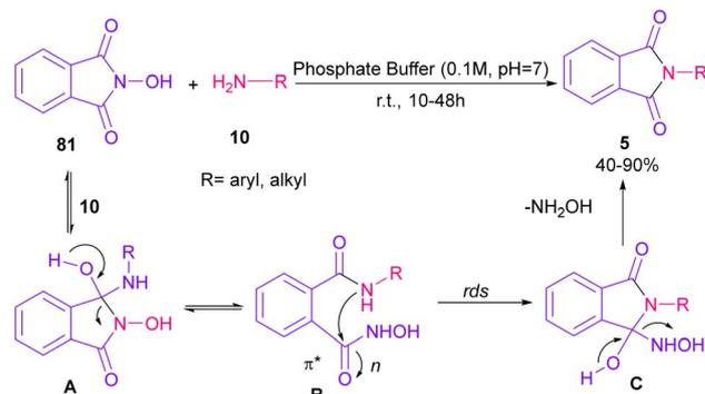
Scheme 55 Phthalimidation of phthalic anhydride by using amines.
