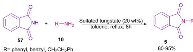
Scheme 50 Sulfated tungstate-catalyzed transamidation of carboxamides with amines.
