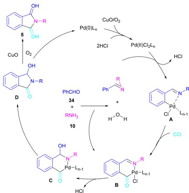
Scheme 22 Possible mechanism for Pd-catalyzed amino-carbonylation of aldehydes.
