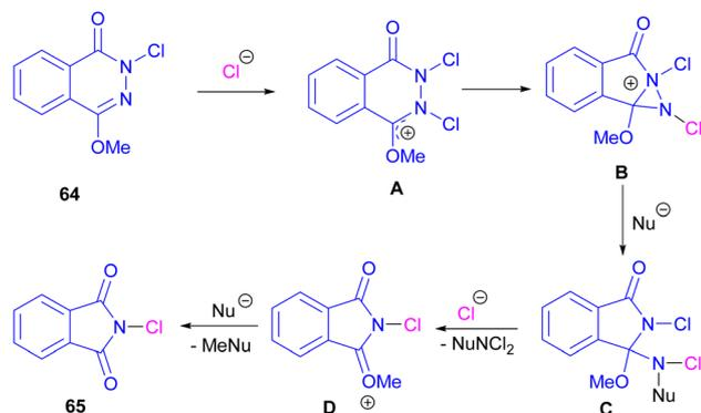
Scheme 44 Plausible mechanism for synthesis of phthalimides from 1,4-dimethoxyphthalazines.
