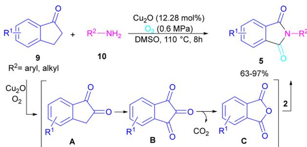
Scheme 5 Cu-catalyzed oxidative reaction of ketones and amines.
