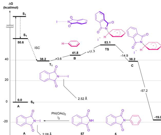
Scheme 59 Proposed mechanism using DFT calculations for visible light-mediated *N*-arylation of phthalimides with arenes.
