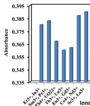
Fig. 4 Effect of 4000 TR of  $Sc^{3+}$ ,  $La^{3+}$ ,  $Sm^{3+}$ ,  $Pr^{3+}$ ,  $Tb^{3+}$ ,  $Lu^{3+}$ ,  $Eu^{3+}$ ,  $Er^{3+}$ ,  $Gd^{3+}$ ,  $Ce^{3+}$ ,  $Nd^{3+}$ ,  $In^{3+}$ ,  $Th^{4+}$ , and  $UO_2^{2+}$  on the absorbance of  $2.5 \times 10^{-7}$  M  $Y^{3+}$  ions using the proposed sensor at the optimum conditions.
