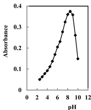
Fig. 2 Effect of pH on the response of the proposed sensor; conditions:  $[Y^{3+}] = 2.5 \times 10^{-7}$  M, membrane cocktail contained 30 mg PVC, 60 mg DMS, 4.0 mg APASA, 2.0 mg TOPO and 3.0 mg Na-TPB.
