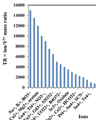
**Fig. 5** Tolerance ratio for various interfering ions in the determination of 2.5 × 10<sup>-7</sup> M of Y<sup>3+</sup>.
