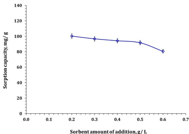
Fig. 12 The effect of Zn/Al-NLDH dose on Zr(IV) uptake (room temperature; 50 mg L<sup>-1</sup> original concentration; 240 min contact time; pH 2.0).
