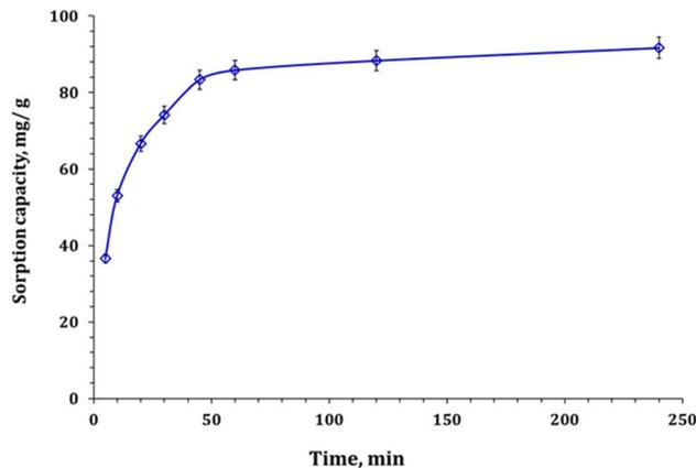
Fig. 7 Zr(IV) sorption capacity as a function of time (pH: 2.0; room temperature; Zr(IV) initial concentration: 50 mg L<sup>-1</sup>; and sorbent dose: 0.5 g L<sup>-1</sup>).
