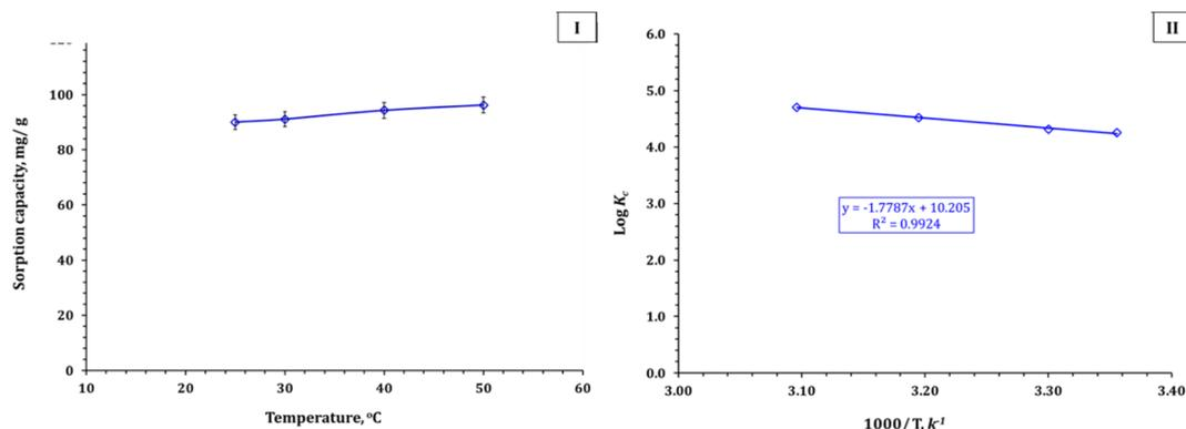
Fig. 13 Effect of sorption temperature on Zr(IV) sorption capacity (I), and Van't Hoff plot for Zr(IV) sorption using Zn/Al-NLDH sorbent (II) (dose 0.5 g L<sup>-1</sup>, shaking time of 120 min, initial concentration 50 mg L<sup>-1</sup>, pH 2.0).
