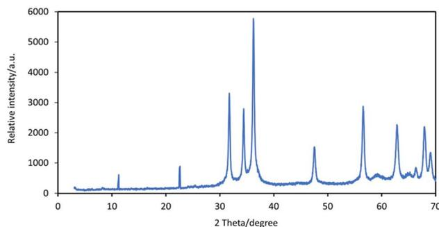
Fig. 2 X-ray diffraction of the prepared NLDH.
