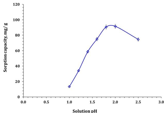
Fig. 6 Zr(IV) sorption capacity as a function of solution pH (mixing time: 120 min; room temperature; Zr(IV) initial concentration: 50 mg L<sup>-1</sup>; and sorbent dose: 0.5 g L<sup>-1</sup>).
