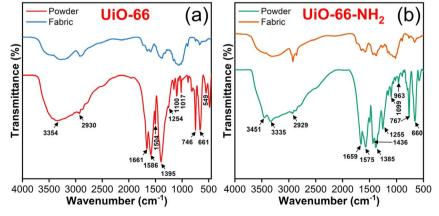
Fig. 5 FTIR spectra of (a) UiO-66 (powder & fabric) and (b) UiO-66-NH<sub>2</sub> (powder & fabric).
