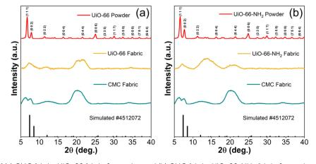
Fig. 2 PXRD patterns of (a) CMC fabric, UiO-66 fabric & powder, and (b) CMC fabric, UiO-66-NH<sub>2</sub> fabric & powder.
