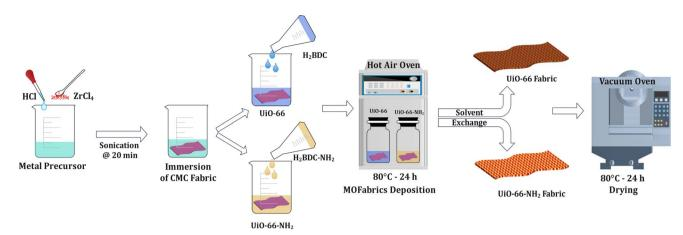
Fig. 1 Solvothermal method to deposit UiO-66 and UiO-66-NH<sub>2</sub> MOFs on cotton fabrics
