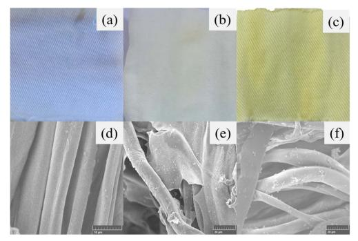
Fig. 3 Photographic and SEM images: ((a) and (d)) CMC fabric, ((b) and (e)) UiO-66 fabric, and ((c) and (f)) UiO-66-NH<sub>2</sub> fabric.
