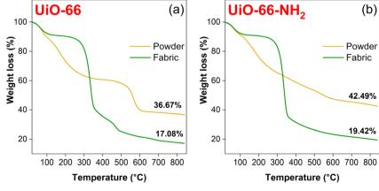
Fig. 6 TGA aerobic curves: (a) UiO-66 (powder & fabric) and (b) UiO-66-NH<sub>2</sub> (powder & fabric) samples.
