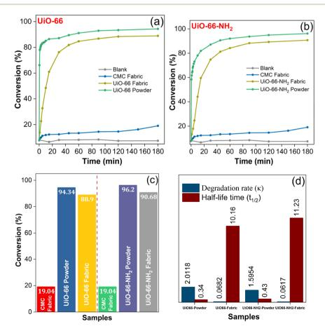
Fig. 7 Catalytic degradation of DMNP to 4-NP as a function of time: (a) UiO-66 (powder & fabric) and (b) UiO-66-NH<sub>2</sub> (powder & fabric), (c) conversion efficiency, and (d) estimated initial rate & half-life.
