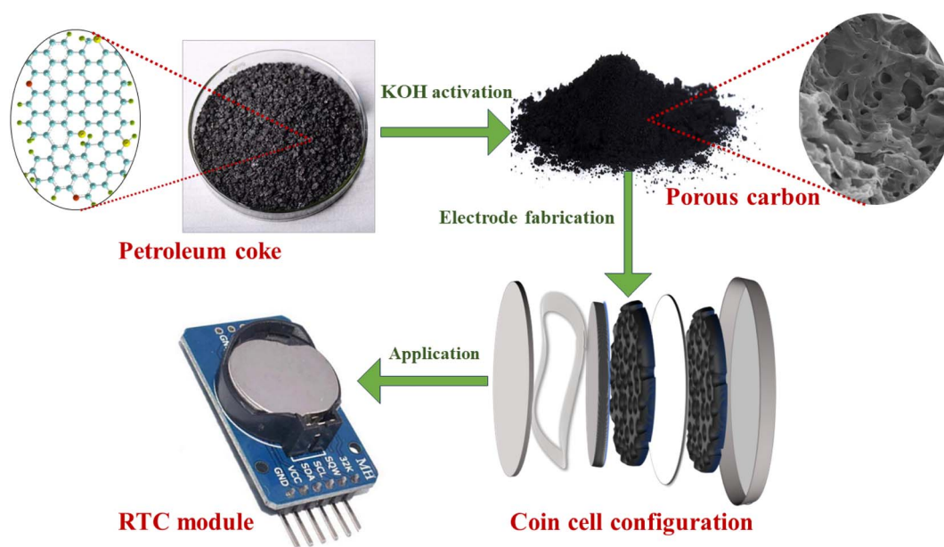
Fig. 1 Schematic representation of the synthesis process, electrode fabrication, and testing of the coin cell supercapacitor in a RTC.
