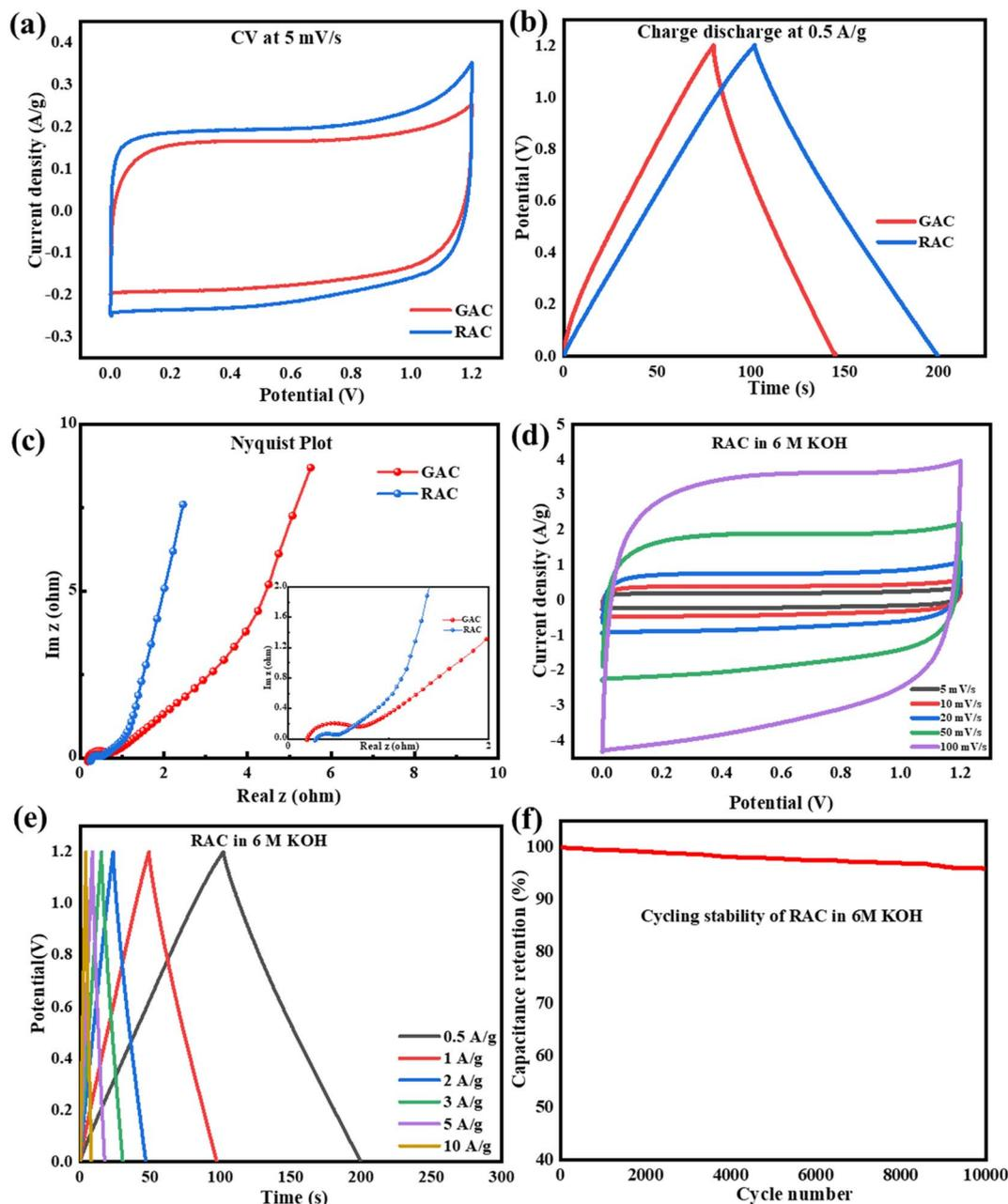
Fig. 7 Electrochemical analysis of pet-coke derived porous carbon in 6 M KOH; (a) comparative CV at a scan rate of  $5 \text{ mV s}^{-1}$ , (b) galvanostatic charge–discharge analysis at  $0.5 \text{ A g}^{-1}$ , (c) Nyquist plot of GAC and RAC showing the resistance performance of the materials, (d) CV analysis of the RAC sample at various scan rates, (e) GCD analysis of the RAC sample at different current densities, and (f) cycling stability of the RAC sample for 10 000 cycles.
