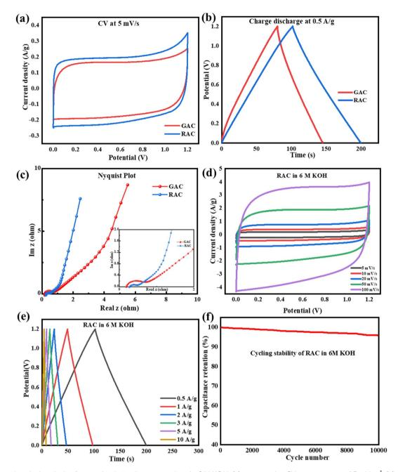
Fig. 7 Electrochemical analysis of pet-coke derived porous carbon in 6 M KOH; (a) comparative CV at a scan rate of 5 mV s $^{-1}$ , (b) galvanostatic charge–discharge analysis at 0.5 A g $^{-1}$ , (c) Nyquist plot of GAC and RAC showing the resistance performance of the materials, (d) CV analysis of the RAC sample at various scan rates, (e) GCD analysis of the RAC sample at different current densities, and (f) cycling stability of the RAC sample for 10 000 cycles.
