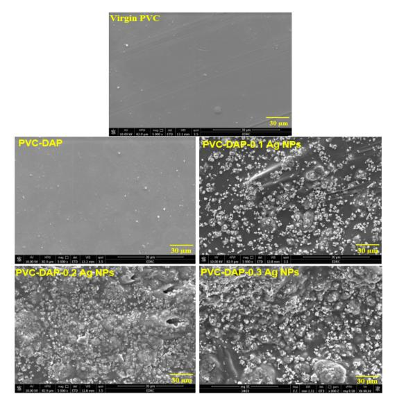
Fig. 5  $\,$  SEM images of virgin PVC, PVC-DAP and the nanocomposites containing various Ag NP proportions after adsorption at 5000imes.
