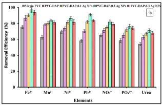
Fig. 4 (a) Schematic representation of the batch adsorption test. (b) Effects of different membranes (virgin PVC, PVC-DAP, PVC-DAP-0.1 Ag NPs, PVC-DAP-0.2 Ag NPs, and PVC-DAP-0.3 Ag NPs) on the removal efficiency of the selected element ions (Fe<sup>3+</sup>, Mn<sup>2+</sup>, Ni<sup>2+</sup>  $Pb^{2+}$ ,  $NO_3^{-}$ ,  $PO_4^{3-}$ , and urea), element ion concentration 10 mg  $L^{-1}$ , pH = 5-7.2 depending the metal ion type, time = 120 min, and adsorbent dose is 3 g  $L^{-1}$ , at 35 °C.
