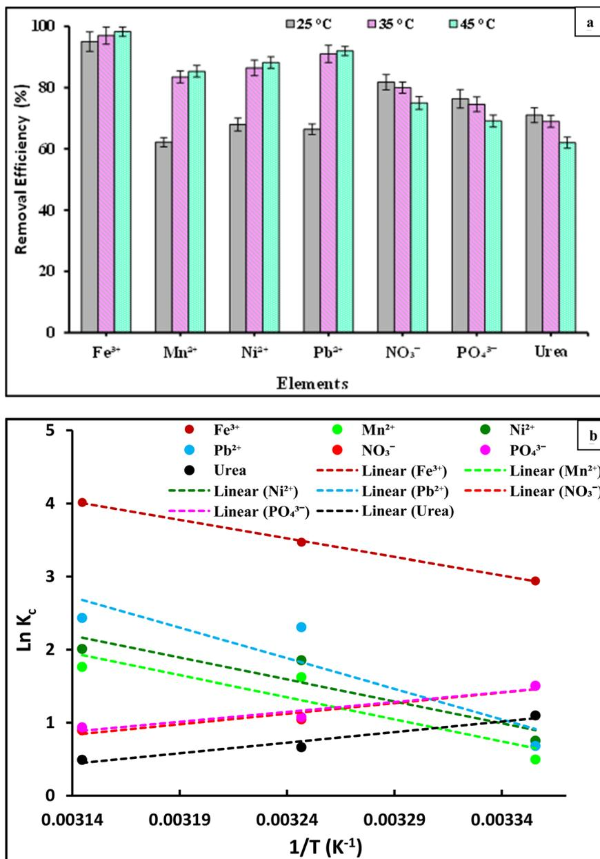
Fig. 8 (a) Effect of temperature; (b) Van't Hoff plot of  $\ln K_c$  versus  $1/T$  for adsorption of  $\text{Fe}^{3+}$ ,  $\text{Mn}^{2+}$ ,  $\text{Ni}^{2+}$ ,  $\text{Pb}^{2+}$ ,  $\text{NO}_3^-$ ,  $\text{PO}_4^{3-}$ , and urea element ions onto the PVC-DAP-0.2 Ag NP membrane, ion concentration  $10 \text{ mg L}^{-1}$ , pH = 5–7.2 according to the type of metal ions, time = 120 min., and adsorbent dose is  $3 \text{ g L}^{-1}$ .
