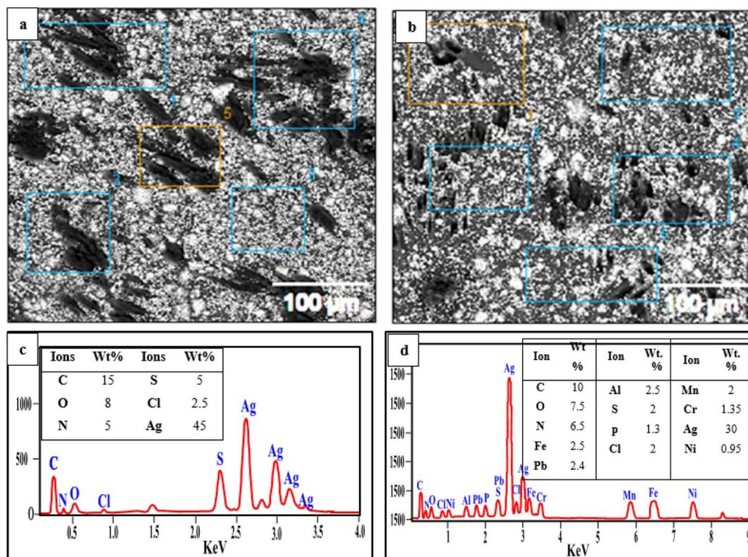
Fig. 10 SEM/EDX analysis before (a and b) and after (c and d) the adsorption of  $\text{Fe}^{3+}$ ,  $\text{Mn}^{2+}$ ,  $\text{Ni}^{2+}$ ,  $\text{Pb}^{2+}$ ,  $\text{NO}_3^-$ ,  $\text{PO}_4^{3-}$ , and urea element ions by the PVC-DAP-0.2 Ag NP membrane.
