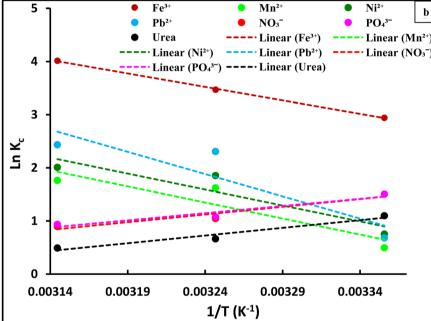
Fig. 8 (a) Effect of temperature; (b) Van't Hoff plot of  $\ln K_c$  versus 1/T for on adsorption of  ${\rm Fe^{3+}}$ ,  ${\rm Mn^{2+}}$ ,  ${\rm Ni^{2+}}$ ,  ${\rm Pb^{2+}}$ ,  ${\rm NO_3^{-}}$ ,  ${\rm PO_4^{3-}}$ , and urea element ions onto the PVC-DAP-0.2 Ag NP membrane, ion concentration 10 mg  ${\rm L^{-1}}$ ,  ${\rm pH}=5-7.2$  according to the type of metal ions, time = 120 min., and adsorbent dose is 3 g  ${\rm L^{-1}}$ .
