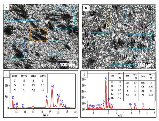
Fig. 10 SEM/EDX analysis before (a and b) and after (c and d) the adsorption of Fe $^{3+}$ , Mn $^{2+}$ , Ni $^{2+}$ , Pb $^{2+}$ , NO $_3^-$ , PO $_4^{3-}$ , and urea element ions by the PVC-DAP-0.2 Ag NP membrane.
