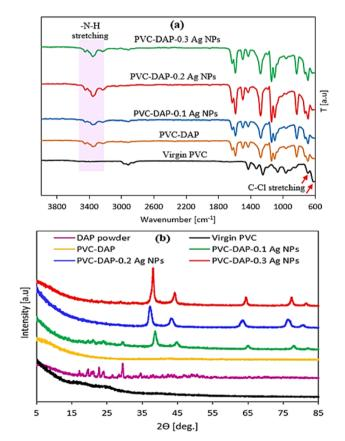
Fig. 3 (a) FTIR spectra of virgin PVC, hybrid PVC, and the nano-composites; (b) XRD patterns of pure DAP, virgin PVC, PVC-DAP, and nonabsorbent films containing varying quantities of Ag NPs.
