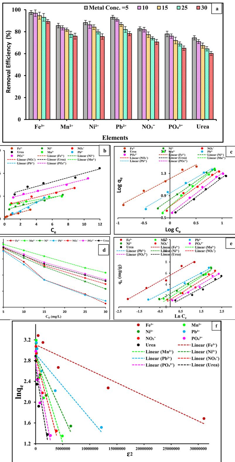
Fig. 7 (a) Effects of element ion concentration (ranging from 5 to 30 mg L<sup>-1</sup>); (b) linearized Langmuir; (c) Freundlich; (d) effect of concentration on Langmuir separation factor; (e) Temkin models; and (f) D-R adsorption isotherm models for Fe<sup>3+</sup>, Mn<sup>2+</sup>, Ni<sup>2+</sup>, Pb<sup>2+</sup>, NO<sub>3</sub><sup>-</sup>, PO<sub>4</sub><sup>3-</sup>, and urea ions onto the PVC-DAP-0.2 Ag NP membrane.
