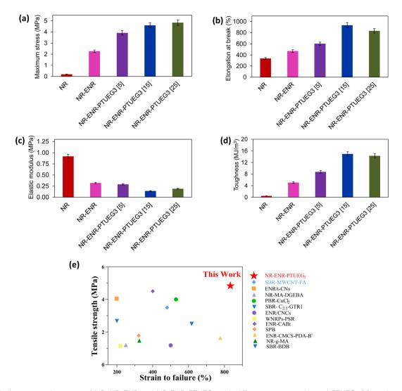
Fig. 3 Typical stress–strain curves of NR, NR-ENR and NR-ENR-PTUEG<sub>3</sub> with different concentrations of PTUEG<sub>3</sub> (a) maximum stress, (b) elongation at break, (c) elastic modulus, (d) toughness, and (e) comparative study between this work and reported self-healing rubber materials. Detailed information is summarized in Table S1.†
