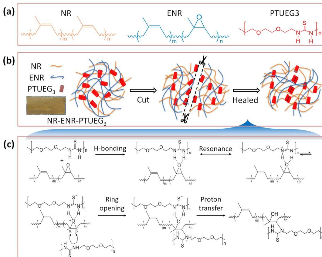
Fig. 1 Mechanism of self-healing rubber NR-ENR-PTUEG<sub>3</sub>. (a) Chemical structure of the component used in the synthesis of NR-ENR-PTUEG<sub>3</sub>. (b) Self-healing mechanism of prepared NR-ENR-PTUEG<sub>3</sub>. (c) Chemical reaction between epoxy and thiourea motif.
