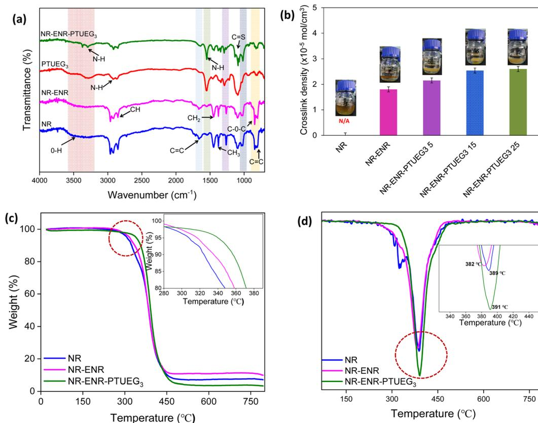
Fig. 2 Characterization of NR-ENR-PTUEG<sub>3</sub>. (a) FTIR spectra of NR, ENR, PTUEG<sub>3</sub> and NR-ENR-PTUEG<sub>3</sub>. (b) Toluene swelling for crosslinking density. (c) TGA curves, and (d) DTG curves.
