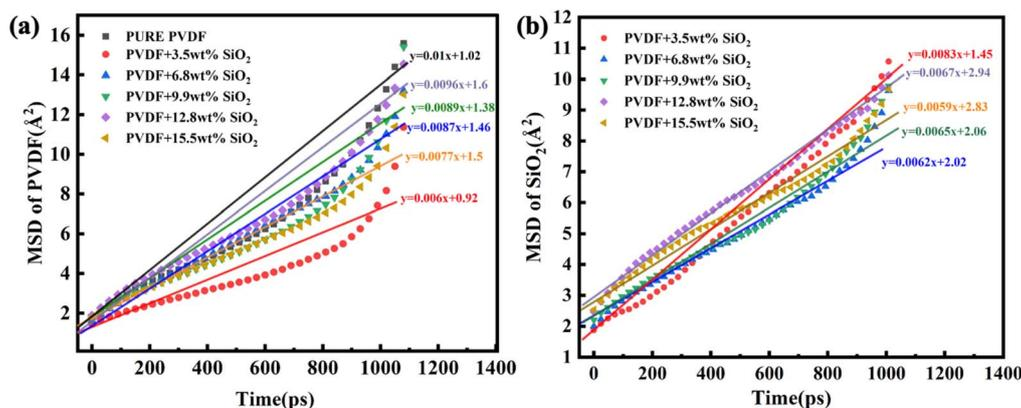
Fig. 2 MSD of PVDF chains (a) and SiO<sub>2</sub> nanoclusters (b).
