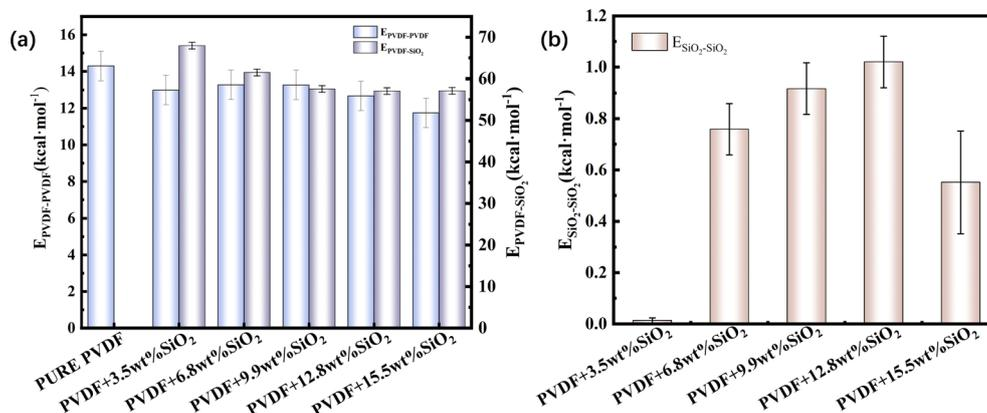
Fig. 4 Interaction energy of PVDF-PVDF, PVDF-SiO<sub>2</sub> (a) and SiO<sub>2</sub>-SiO<sub>2</sub> (b).
