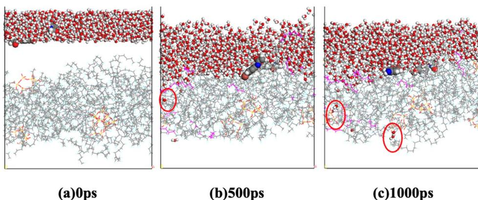
Fig. 11 Diffusion process of lubricating-water on the PVDF membrane with a 3.5 wt% addition of  $\text{SiO}_2$  for different time intervals: (a) 0 ps, (b) 500 ps, and (c) 1000 ps. Water is represented using a ball and stick model, membranes are depicted using a line model, and oil is represented using a CPK model.
