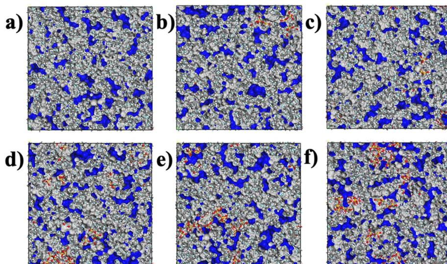
Fig. 6 Free volume inside the SiO<sub>2</sub>/PVDF membranes: (a) pure PVDF, (b) PVDF + 3.5 wt% SiO<sub>2</sub>, (c) PVDF + 6.8 wt% SiO<sub>2</sub>, (d) PVDF + 9.9 wt% SiO<sub>2</sub>, (e) PVDF + 12.8 wt% SiO<sub>2</sub>, (f) PVDF + 15.5 wt% SiO<sub>2</sub>. The blue denotes the area of free volume. Via the hardsphere probe method, the probe radius ( $R_p$ ) = 0.5.
