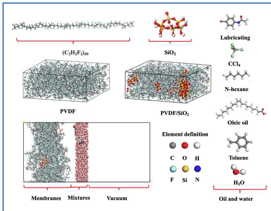
Fig. 1 Models of the PVDF, SiO<sub>2</sub>/PVDF and oil molecules.
