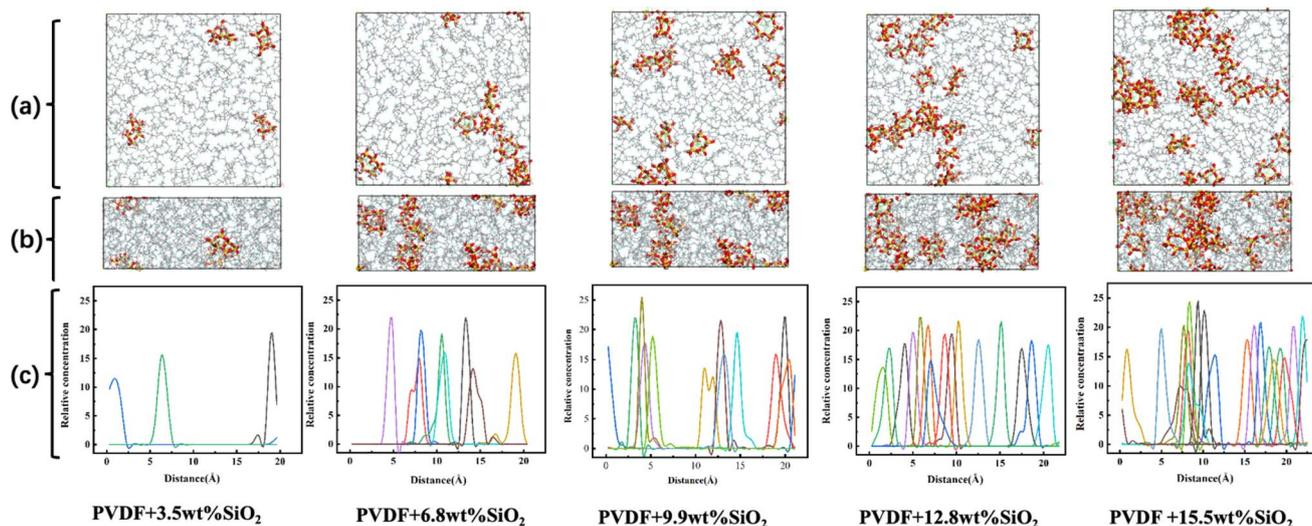
Fig. 3 The distribution of SiO<sub>2</sub> nanoparticles in hybrid membranes along the Z-axis. (a) Top view, (b) side view, (c) relative concentration profiles (each color curve represents a different SiO<sub>2</sub> cluster in the membrane).
