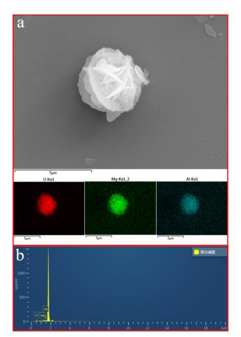
Fig. 3 (a) Elemental mapping characterization of prepared MgAl-LDH nanoflower. (b) EDS profile obtained from MgAl-LDH nanoflower.
