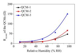
Fig. 7 The change in  $R_{\rm crystal}$  of QCM-1, QCM-2, and QCM-3 as a function of humidity.
