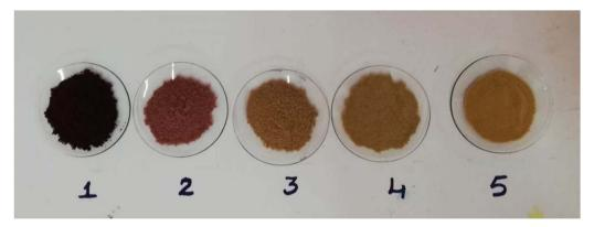
Fig. 26 : Powders 1 to 4: fresh samples of NICSS added to AR119-TIE solution after every 15 min, filtered and the residue dried in an oven. Sample 5: NICSS.
