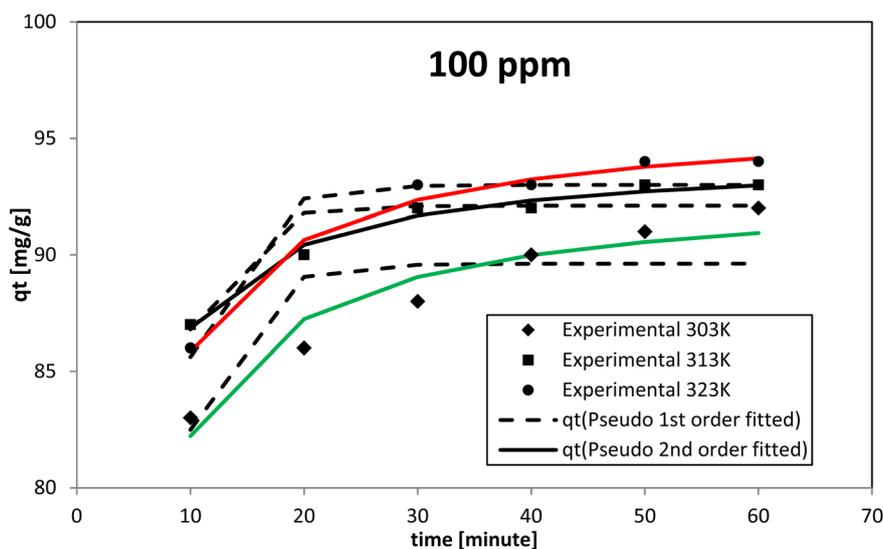
Fig. 13 Adjustments of kinetic models to an initial concentration of 100 ppm.
