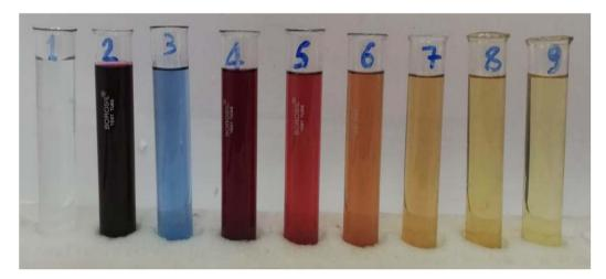
Fig. 27 Color of the solutions before and after adsorption. (1) Distilled water; (2) AR119 in distilled water; (3) TIE; (4) AR119 in TIE; (5) filtrate after adsorption of dye on NICSS after 15 min; (6) 30 min; (7) 45 min; (8) 60 min; (9) filtrate of NICSS in distilled water.
