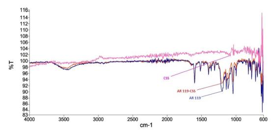
Fig. 3 FTIR spectroscopy ranges of AR119 dye, NICSS and AR119 dye adsorbed on NICSS.
