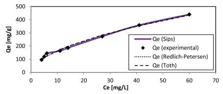
Fig. 12 Sips, Redlich-Petersen, and Toth adsorption isotherms.
