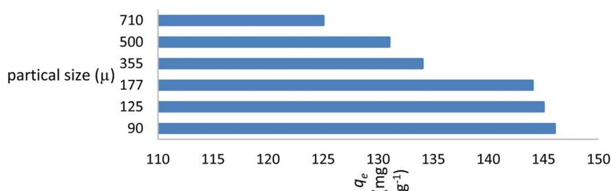
Fig. 7 Impact of the size of adsorbent particles.
