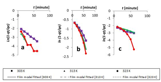
Fig. 18 Kinetics data, with an initial concentration of AR119, were modeled according to the film diffusion model: (a) 100 ppm, (b) 150 ppm and (c) 200 ppm.
