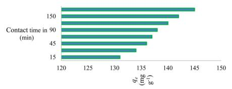
Fig. 8 Influence of exposure time on dye adsorption.
