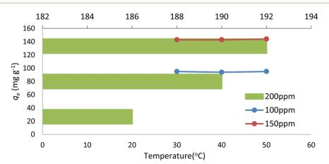
Fig. 9 Impact of temperature on dye adsorption.
