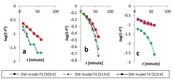
Fig. 16 Kinetics data, beginning with an initial concentration of AR119, was modeled according to the Dumwald-Wagner model: (a) 100 ppm, (b) 150 ppm and (c) 200 ppm.
