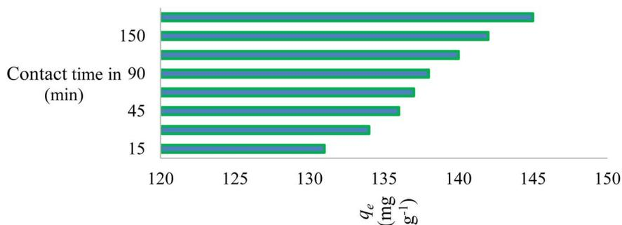
Fig. 8 Influence of exposure time on dye adsorption.
