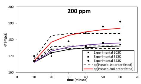
Fits of kinetic models for an initial concentration of 200 ppm.
