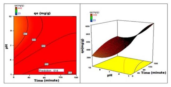
Fig. 24 Variation in the adsorption capability with time in connection to pH.
