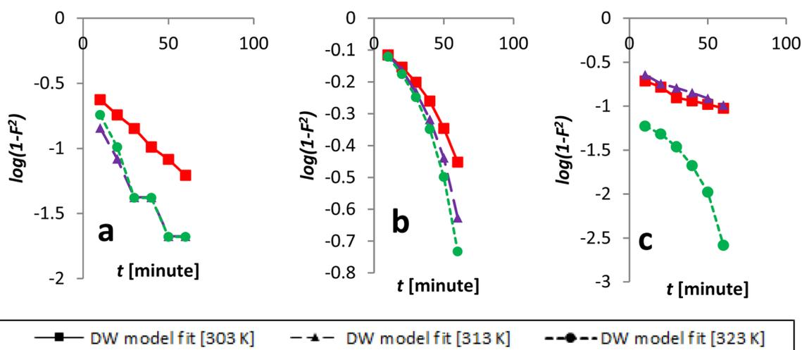
Fig. 16 Kinetics data, beginning with an initial concentration of AR119, was modeled according to the Dumwald–Wagner model: (a) 100 ppm, (b) 150 ppm and (c) 200 ppm.
