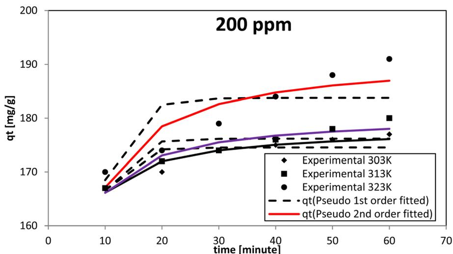
Fig. 15 Fits of kinetic models for an initial concentration of 200 ppm.
