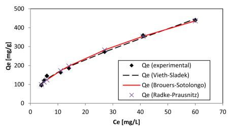
Fig. 11 Adsorption isotherms of Vieth-Sladek, Brouers-Sotologgo, and Radke-Prausnitz.
