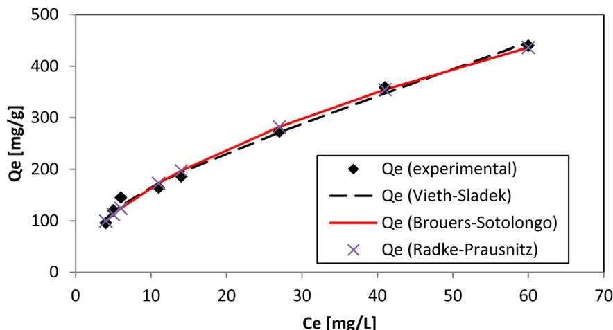
Fig. 11 Adsorption isotherms of Vieth–Sladek, Brouers–Sotolongo, and Radke–Prausnitz.
