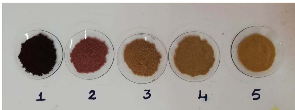
Fig. 26 : Powders 1 to 4: fresh samples of NICSS added to AR119-TIE solution after every 15 min, filtered and the residue dried in an oven. Sample 5: NICSS.
