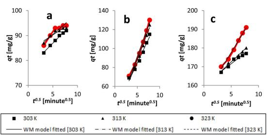
Fig. 17 Kinetics data, with an initial concentration of AR119, were analyzed using the Weber-Morris model: (a) 100 ppm, (b) 150 ppm and (c) 200 ppm.
