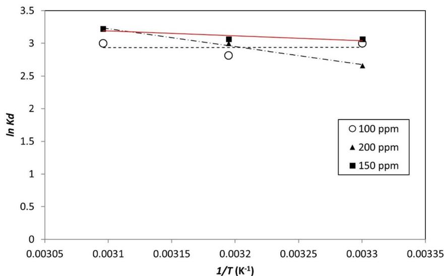
Fig. 19 Plotting the thermodynamic equilibrium constant versus the reciprocal of temperature ( $1/T$ ), the enthalpy and Gibbs free energy of the process was determined.
