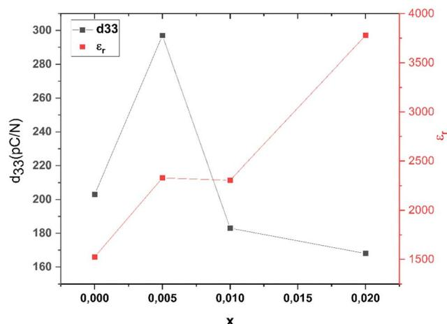
**Fig. 12** The relative dielectric constant  $\varepsilon_r$  at room temperature (100 Hz) and piezoelectric coefficient  $d_{33}$  of the BCZT–xZT ceramics.
