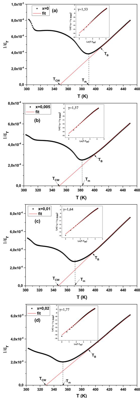
Fig. 10 Inverse dielectric constant at 1 kHz as a function of temperature for the BCZT-*x*ZT ceramics. The inset shows the  $\log\left(\frac{1}{\epsilon_r} - \frac{1}{\epsilon_m}\right)$  against  $\log(T - T_m)$  at 1 kHz.
