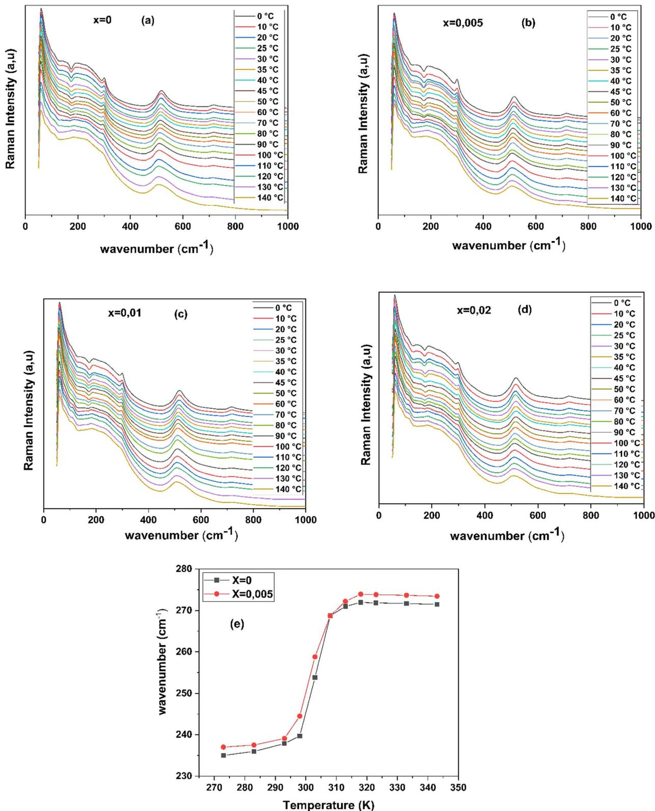
Fig. 7 (a–d) Temperature evolution of Raman spectra of BCZT–xZT in vicinity of orthorhombic-to-tetragonal phase transition during heating and (e) frequency of A(TO<sub>2</sub>) mode as a function of temperature.
