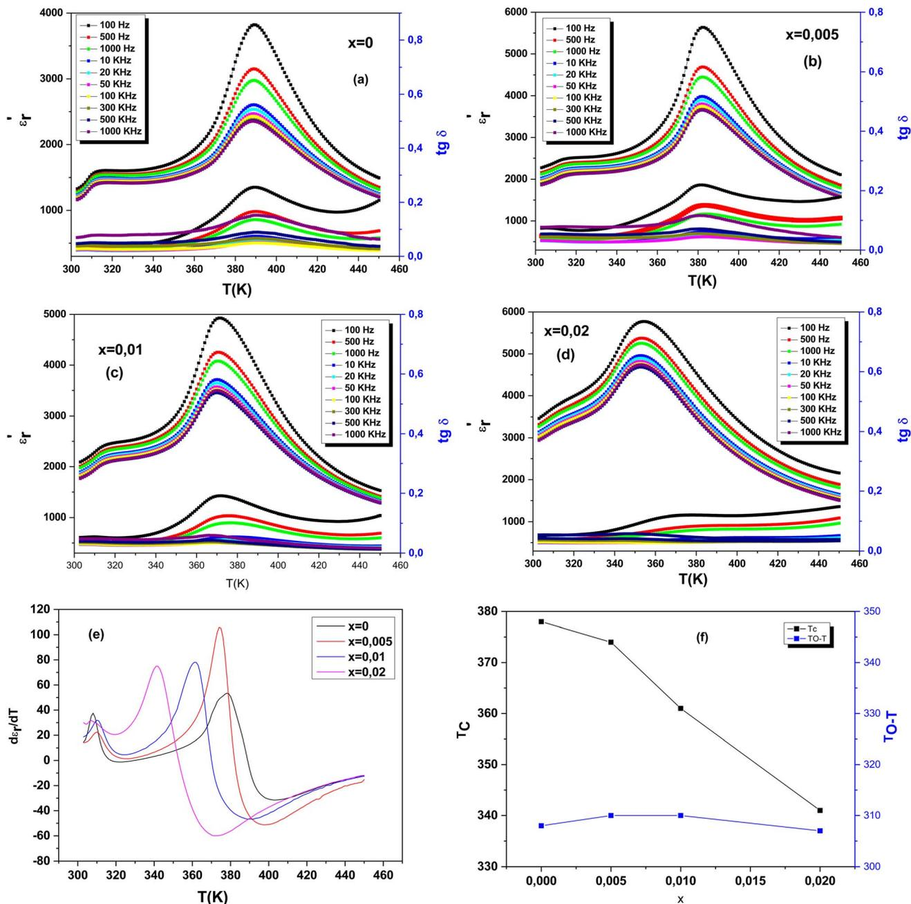
Fig. 8 (a)–(d) Temperature dependence of the dielectric constant of BCZT-xBZT ceramics: (a)  $x = 0$ , (b)  $x = 0.005$ , (c)  $x = 0.01$ , (d)  $x = 0.02$ ; (e) the derivative of the dielectric constant as a function of temperature for each composition; (f) phase diagram of BCZT-xZT based on the present dielectric measurements.
