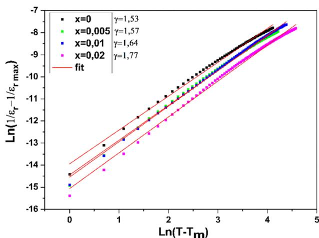
**Fig. 11** The  $\log\left(\frac{1}{\varepsilon_r} - \frac{1}{\varepsilon_m}\right)$  against  $\log(T - T_m)$  at 1 kHz for BCZT–xBZT ceramics.
