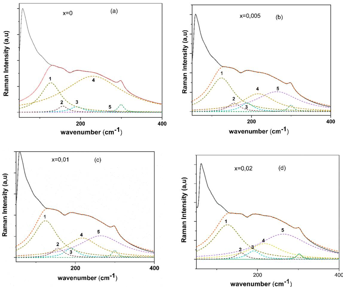
Fig. 6 (a–d) Room temperature Raman spectra of BCZT-xZT in the range (a) 50 to 300  $\text{cm}^{-1}$  along with spectra de-convolution.
