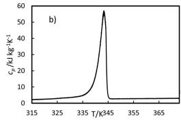
Fig. 4 Experimental enthalpies, h (a) and heat capacity,  $c_p$  (b) versus temperature, T, for OM65 at 0.5 K min<sup>-1</sup>. The solid line is the heating cycle, and the dashed line is the cooling cycle.
