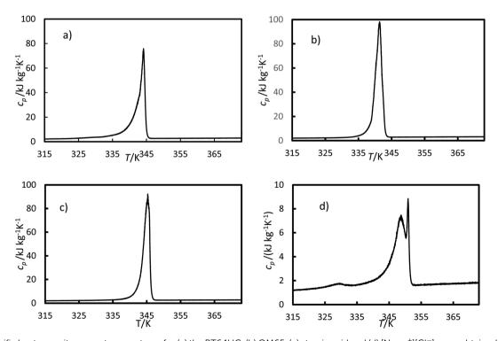
Fig. 10 Specific heat capacity versus temperatures for (a) the RT64HC, (b) OM65, (c) stearic acid and (d) [N<sub>4444</sub><sup>+</sup>][Cl<sup>-</sup>] were obtained using eqn (5) and data from the DSC measurement.
