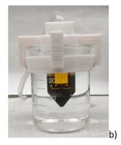
Fig. 6 Thermal conductivity sensors for (a) the solid sample and (b) liquid sample including the support to hold the sensor.
