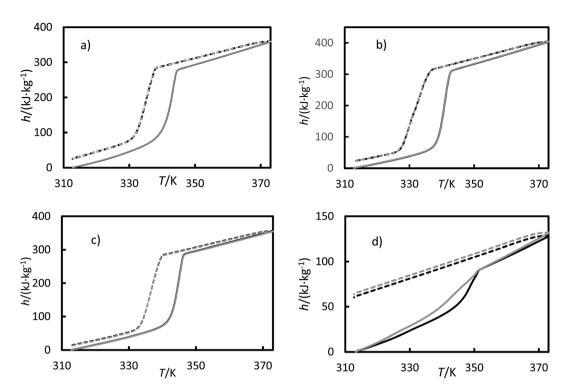
Fig. 9 Enthalpies versus temperatures for (a) the RT64HC, (b) OM65, (c) stearic acid and (d) [N<sub>4444</sub><sup>+</sup>][Cl<sup>-</sup>] from a DSC measurement. Solid curves represent the heating ramp, and the dashed line represents the cooling ramp. Black represents the second cycle, and gray represents the third cycle.
