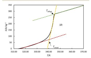
Fig. 5 Experimental enthalpies *versus* temperature for OM65 at 0.5 K min $^{-1}$ . An example of determining the onset and offset temperatures,  $T_{\rm onset}$  and  $T_{\rm offset}$  and phase transition enthalpy,  $\Delta h$ .
