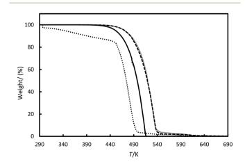
Fig. 8 Thermogravimetric analysis (TGA) for the (–) OM65, (–) RT64H, (grey line) stearic acid and  $(\cdots)$  [N<sub>4444</sub><sup>+</sup>][Cl<sup>-</sup>].
