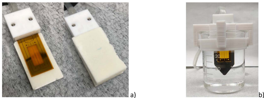
Fig. 6 Thermal conductivity sensors for (a) the solid sample and (b) liquid sample including the support to hold the sensor.
