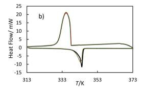
Fig. 3 Thermogram of OM65 at 0.5 K min<sup>-1</sup> obtained by hf-DSC; (a) heat flow *versus* time for one cycle and (b) heat flow *versus* temperature for three cycles: black line, cycle 1; red line, cycle 2; and green line cycle 3.
