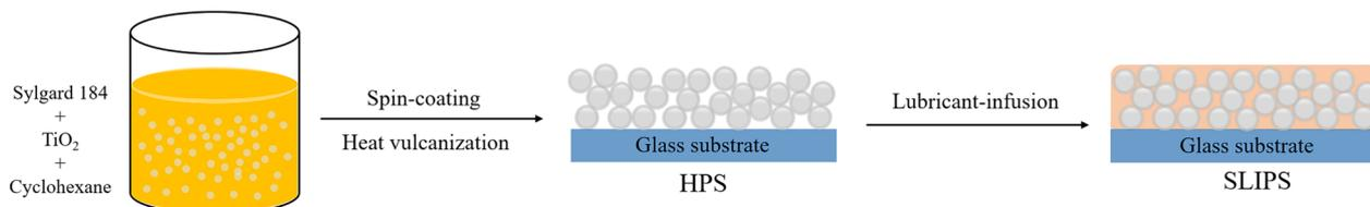
Fig. 1 Schematic for the preparation of the SLIPS.
