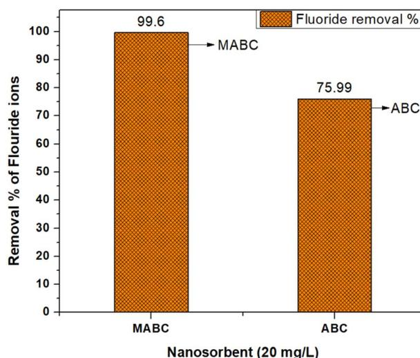
Fig. 13 Comparative fluoride adsorption using MABC and ABC.
