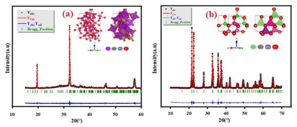
Fig. 2 XRD patterns of as-prepared (a) K<sub>2</sub>ZnGeO<sub>4</sub> and (b) Li<sub>2</sub>ZnGeO<sub>4</sub> compounds
