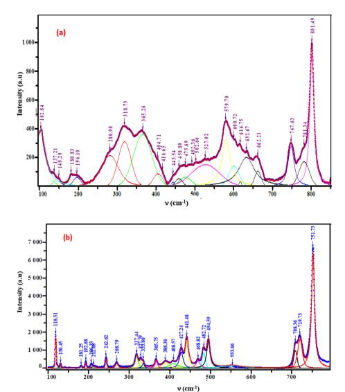
Fig. 5 Raman spectra of the phosphors (a)  $K_2ZnGeO_4$ , (b)  $Li_2ZnGeO_4$ .
