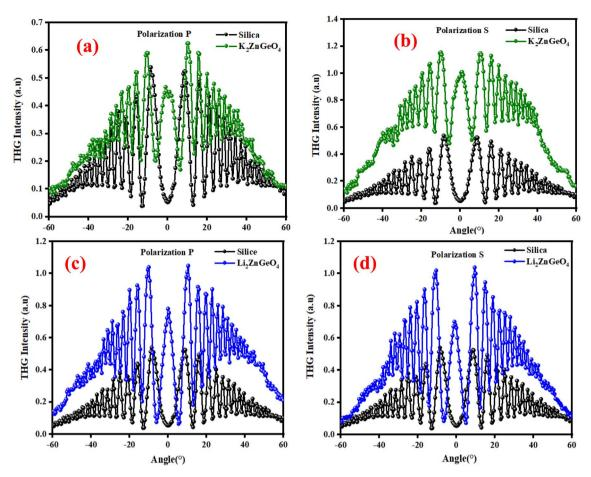
Fig. 16 Third harmonic intensity plotted against the incident angle for polarization P and S of  $K_2ZnGeO_4$  film and silica (a) and (b) and  $Li_2ZnGeO_4$  film and silica (c) and (d).
