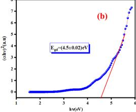
Fig. 7 Plots of  $(\alpha h\nu)^2$  as a function as  $h\nu$  of (a)  $K_2ZnGeO_4$  and (b)  $Li_2ZnGeO_4$
