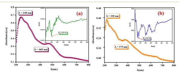
Fig. 6 The UV-vis absorbance spectrum A ( $\lambda$ ) and  $dA/d\lambda$  as a function of  $\lambda$  in the inset for the phosphors  $K_2ZnGeO_4$  (a) and  $Li_2ZnGeO_4$  (b) at room temperature, spanning from 200 to 800 nm.
