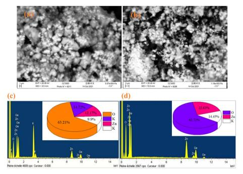
$Fig. \ 3 \quad \text{SEM image of } K_2ZnGeO_4 \ (a) \ \text{and } Li_2ZnGeO_4 \ (b), \ \text{along with the elemental analysis by EDX of } K_2ZnGeO_4 \ (c) \ \text{and } Li_2ZnGeO_4 \ (d).$
