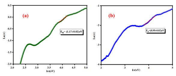
Fig. 9 Determining the Urbach energy of the (a) K<sub>2</sub>ZnGeO<sub>4</sub> and (b) Li<sub>2</sub>ZnGeO<sub>4</sub>.
