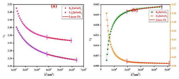
Fig. 14 (a) The variation of  $\varepsilon_1$  with  $\lambda_2$  and (b) The  $\varepsilon_2$  against  $\lambda^3$  for the A<sub>2</sub>ZnGeO<sub>4</sub> (K, Li).
