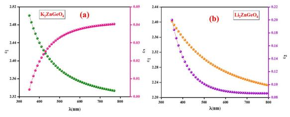
Fig. 13 The  $\varepsilon_1$  and  $\varepsilon_2$  against the  $\lambda$  of the (a) K<sub>2</sub>ZnGeO<sub>4</sub> and (b) Li<sub>2</sub>ZnGeO<sub>4</sub>.
