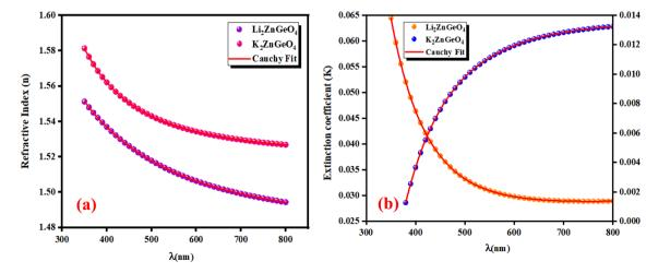
Fig. 10 Refractive index (a) and extinction coefficient (b) plots versus wavelength for K<sub>2</sub>ZnGeO<sub>4</sub> and Li<sub>2</sub>ZnGeO<sub>4</sub> compounds.
