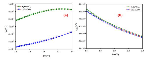
Fig. 15 (a) The variation of the optical conductivity and (b) the electrical conductivity versus the photon energy for the  $A_2ZnGeO_4$  thin films.
