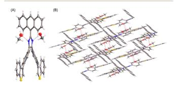
Fig. 6 (A) ORTEP drawing (at 50% ellipsoid probability) of the molecular structure of **5b** solvate determined by single-crystal X-ray diffraction analysis. (B) Packing motif shown in the crystal structure of **5b** solvate. CCDC 2354150.
