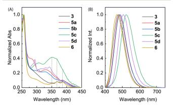
Fig. 7 (A) Normalized UV-Vis absorption and (B) normalized fluorescence spectra ( $\lambda_{\rm ex} = 360$  nm) of compounds **3**, **5a–d**, and **6** measured in CH<sub>2</sub>Cl<sub>2</sub> at room temperature.
