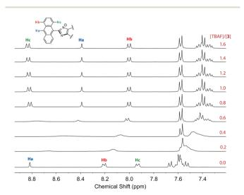
Fig. 15  $^{1}$ H NMR (300 MHz, DMSO- $d_{6}$ ) titration of 3 (3.61 mM) with TBAF (0 to 2.2 mole equiv.) at room temperature.
