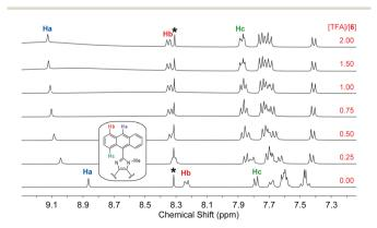
Fig. 11  $^{1}$ H NMR (300 MHz, DMSO- $d_{\rm c}$ ) titration of **6** (5.57 mM) with TFA (0 to 2.0 mole equiv.) at room temperature. The singlet at 8.30 ppm (labelled by \*) is due to residual DMF in the solution.
