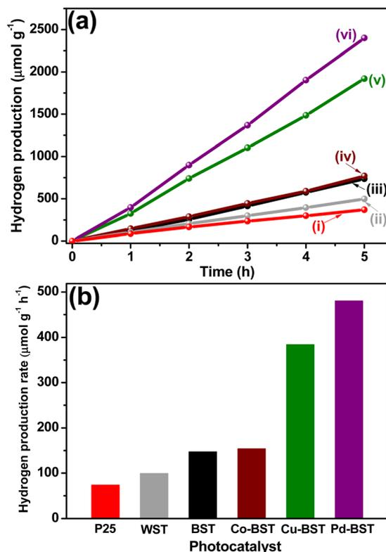
Fig. 7 (a) Hydrogen generation of: (i) Degussa P<sub>25</sub>, (ii) WST, (iii) BST, (iv) Co-BST, (v) Cu-BST and (vi) Pd-BST and (b) hydrogen generation rate of structures with co-catalyst.
