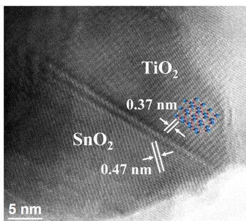
Fig. 2 HR-TEM image of black  $\text{SnO}_2$ - $\text{TiO}_2$  structure.
