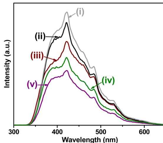
Fig. 11 PL spectra of: (i) white  $SnO_2-TiO_2$  (WST), (ii) black  $SnO_2-TiO_2$  (BST), (iii) Co-BST, (iv) Cu-BST and (v) Pd-BST.
