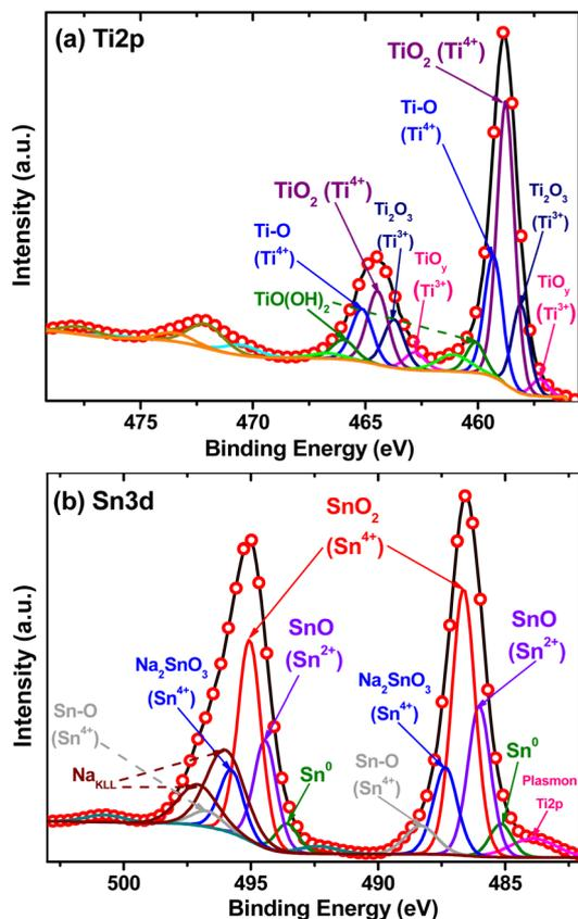
Fig. 5 XPS high-resolution spectra of: (a) Ti 2p region and (b) Sn 3d region for black SnO<sub>2</sub>-TiO<sub>2</sub> structure.
