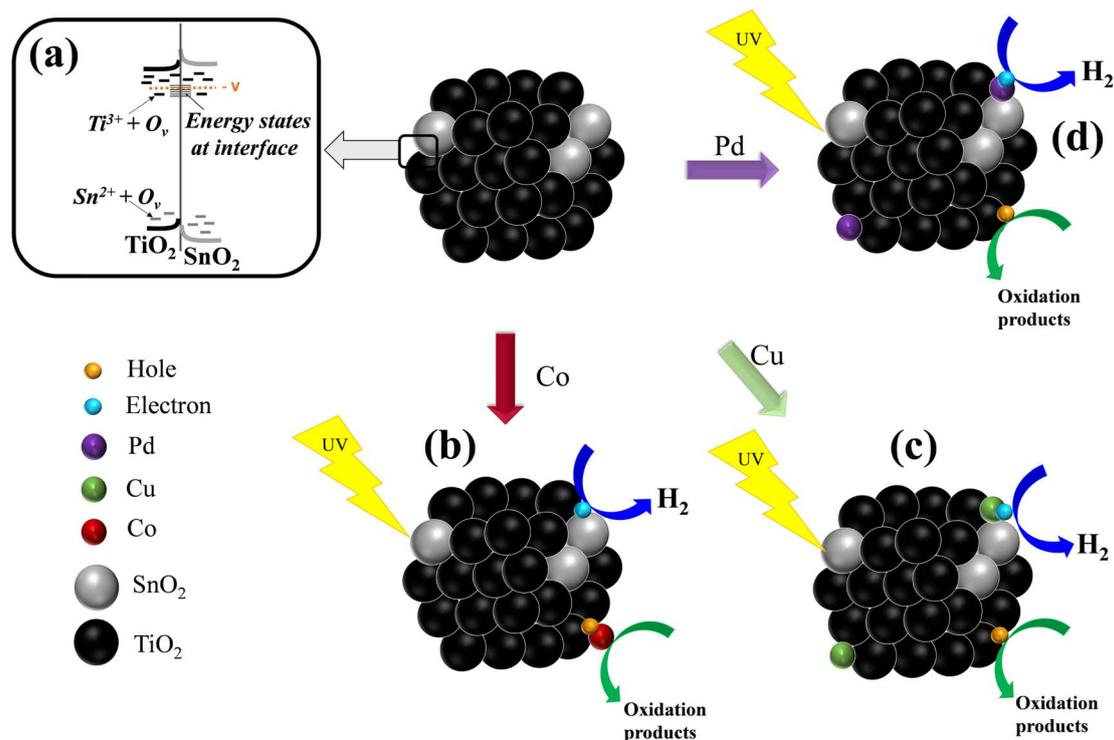
Scheme 1 Representation of the mobility, separation and charge transfer in: (a) black  $\text{SnO}_2\text{-TiO}_2$  structure, (b) black  $\text{SnO}_2\text{-TiO}_2$  with cobalt species, (c) black  $\text{SnO}_2\text{-TiO}_2$  with copper species and (d) black  $\text{SnO}_2\text{-TiO}_2$  with palladium species for photocatalytic hydrogen generation.
