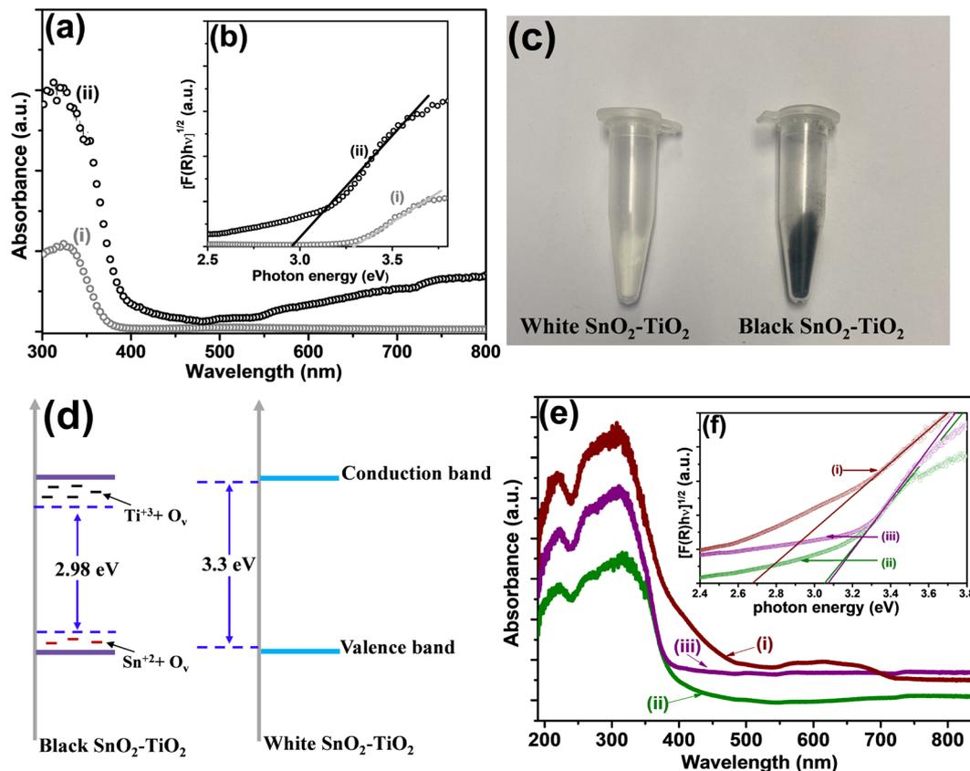
Fig. 3 (a) UV-visible spectra of: (i) WST and (ii) BST, (b) insert of the bandgap energy ( $E_g$ ) estimation of: (i) WST and (ii) BST, (c) images of white and black  $\text{SnO}_2\text{-TiO}_2$  powders. (d) schematic diagram of WST and BST (the presence of  $\text{Ti}^{3+}$  and  $\text{Sn}^{2+}$  states), (e) UV-visible spectra of: (i) Co-BST, (ii) Cu-BST and (iii) Pd-BST and (f) insert of the bandgap energy ( $E_g$ ) estimation of: (i) Co-BST, (ii) Cu-BST and (iii) Pd-BST.
