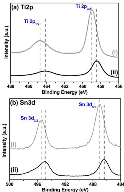
Fig. 4 XPS high resolution spectra of (a) Ti 2p energy zone of: (i) white SnO<sub>2</sub>-TiO<sub>2</sub> (WST) and (ii) black SnO<sub>2</sub>-TiO<sub>2</sub> (BST), and XPS high resolution spectra of (b) Sn 3d energy zone of: (i) white SnO<sub>2</sub>-TiO<sub>2</sub> (WST) and (ii) black SnO<sub>2</sub>-TiO<sub>2</sub> (BST).
