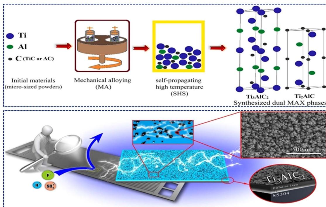
Fig. 17 Schematic representation illustrating the synthesis process of low-cost  $\text{Ti}_3\text{AlC}_2$ - $\text{Ti}_2\text{AlC}$  dual MAX phase, highlighting the use of economical raw materials and innovative compositions for achieving high-electrical conductivity. (Reproduced from ref. 288 with permission from Elsevier, copyright 2023).<sup>288</sup> (Reproduced from ref. 289 with permission from Elsevier, copyright 2019).<sup>289</sup>
