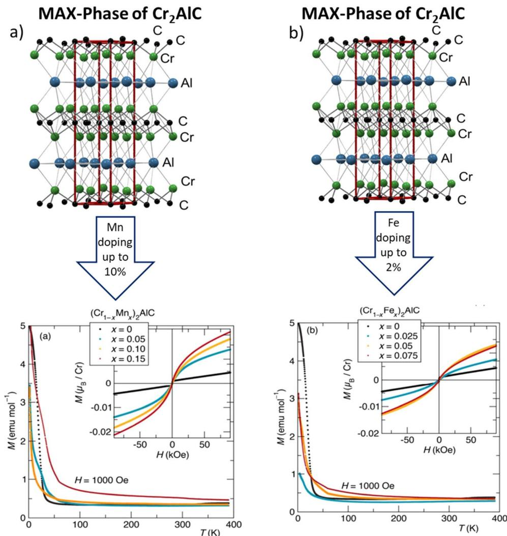
Fig. 10 Magnetization data for the Mn (a) and Fe (b) substituted samples,  $(\text{Cr}_{1-x}\text{Mn}_x)_2\text{AlC}$  and  $(\text{Cr}_{1-x}\text{Fe}_x)_2\text{AlC}$ , with nominal compositions. (Reproduced from ref. 209 with permission from The Royal Society of Chemistry, copyright 2017).<sup>209</sup>
