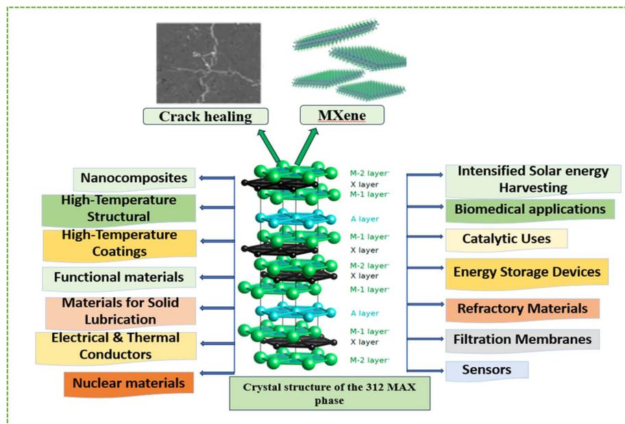
Fig. 13 The overview of multi-applications of MAX-phases.
