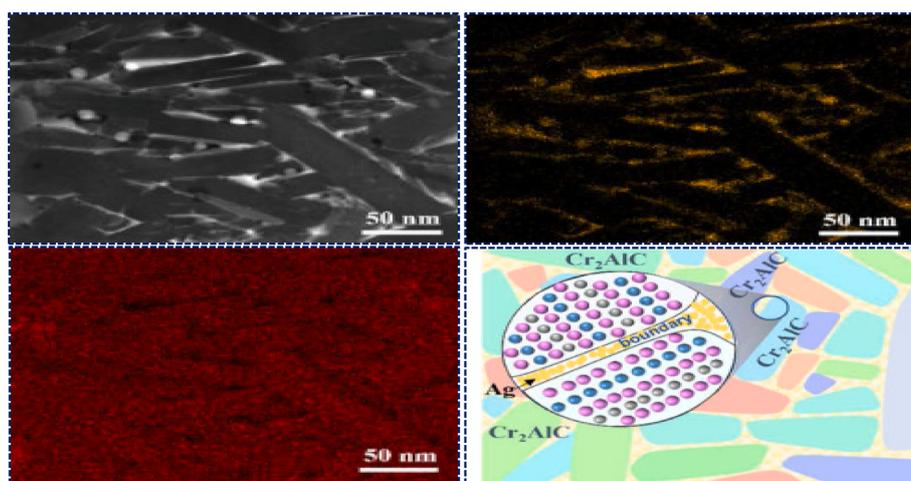
Fig. 16 The cross-sectional images and schematics representation of the Ag doped  $\text{Cr}_2\text{AlC}$  nanocomposite coatings. (Reproduced from ref. 283 with permission from Elsevier, copyright 2024).<sup>283</sup>
