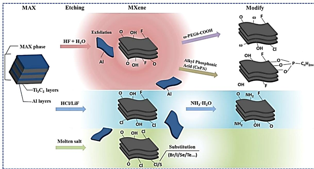
Fig. 20 The prevailing method for producing MXene currently. (Reproduced from ref. 305 with permission from MDPI AG, copyright 2022).<sup>305</sup>
