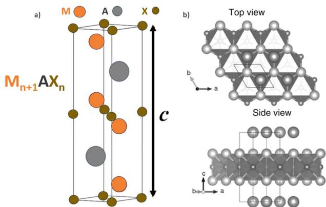
Fig. 2 (a) Unit cell and (b) crystal structure of MAX-phases. (Reproduced from ref. 72 with permission from American Physical Society, copyright 2004).<sup>72</sup>
