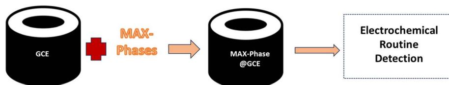
Fig. 24 Schematic of MAX-phase integration with Glassy Carbon Electrode (GCE) for enhanced performance as a sensor. (Reproduced from ref. 328 with permission from Elsevier, copyright 2022).<sup>328</sup>
