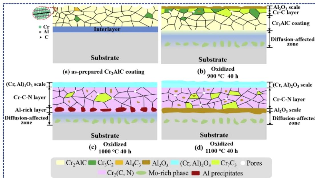
Fig. 15 Oxidation mechanisms of Cr<sub>2</sub>AlC MAX phase coatings at 900–1100 °C. (Reproduced from ref. 277 with permission from Elsevier, copyright 2020).<sup>277</sup>
