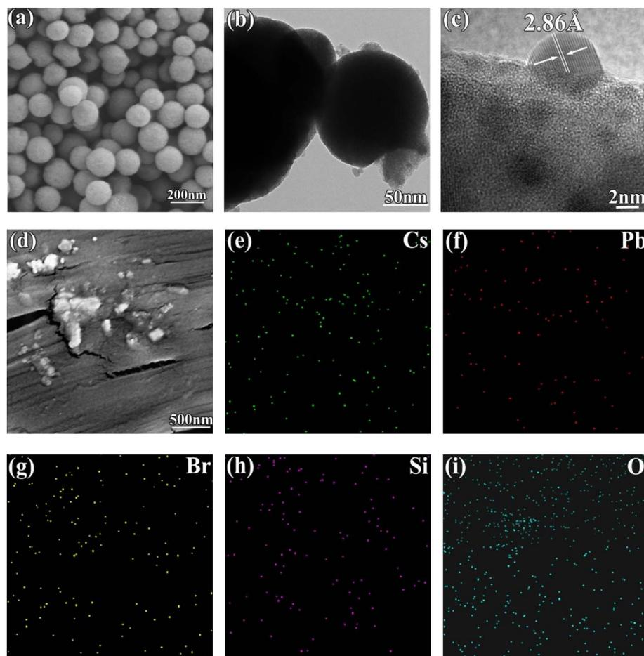
Fig. 2 (a) SEM image of  $m\text{-SiO}_2$ , (b) TEM image of  $m\text{-SiO}_2/\text{CsPbBr}_3$  composites, (c) HRTEM image of  $m\text{-SiO}_2/\text{CsPbBr}_3$  composites, (d) SEM image of  $\text{PMMA}@m\text{-SiO}_2/\text{CsPbBr}_3$  composite luminescent device, (e) EDS energy spectra of Cs, (f) Pb, (g) Br, (h) Si and (i) O in  $\text{PMMA}@m\text{-SiO}_2/\text{CsPbBr}_3$  flexible film.
