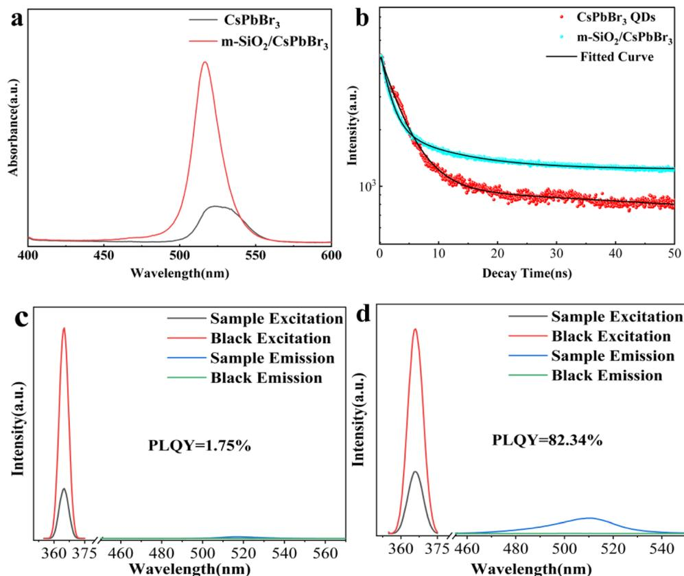
Fig. 3 (a) PL spectrum of CsPbBr<sub>3</sub> QDs and m-SiO<sub>2</sub>/CsPbBr<sub>3</sub> composites. (b) Fluorescence lifetime decay curves of CsPbBr<sub>3</sub> QDs and m-SiO<sub>2</sub>/CsPbBr<sub>3</sub> composites. (c) PLQY plot of CsPbBr<sub>3</sub> QDs (d) PLQY plot of m-SiO<sub>2</sub>/CsPbBr<sub>3</sub> composites.
