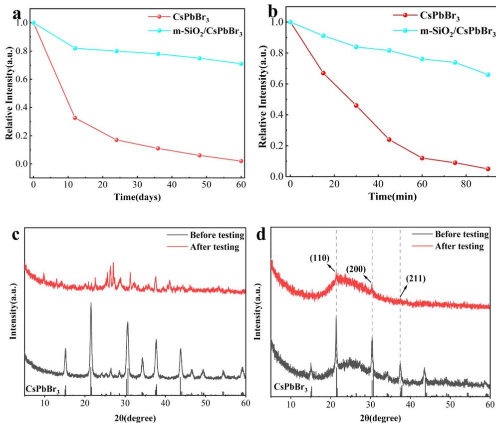
Fig. 4 (a) Storage stability of CsPbBr<sub>3</sub> QDs and m-SiO<sub>2</sub>/CsPbBr<sub>3</sub> composites. (b) Water stability of CsPbBr<sub>3</sub> QDs and m-SiO<sub>2</sub>/CsPbBr<sub>3</sub> composites. (c) Phase stability of CsPbBr<sub>3</sub> QDs and (d) m-SiO<sub>2</sub>/CsPbBr<sub>3</sub> composites.
