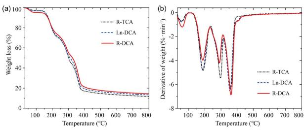
Fig. 4 TG (a) and DTG (b) curves of chitin aerogels under nitrogen atmosphere.
