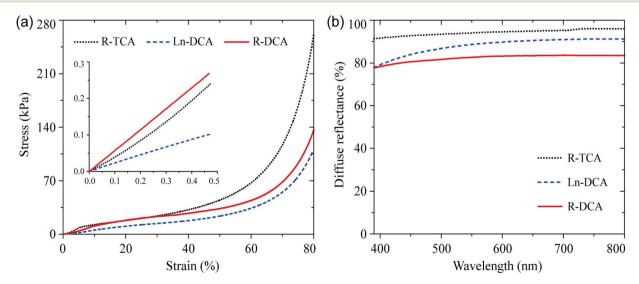
Fig. 6 (a) Compression stress-strain curves of chitin aerogels. Insert shows the typical elastic deformation region. (b) Diffuse reflectance of chitin aerogels within the visible light region.
