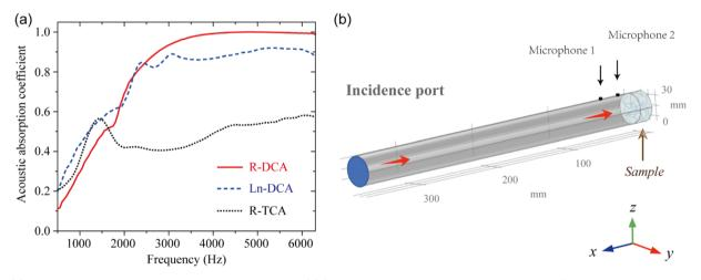
Fig. 5 (a) Acoustic absorption performance of chitin aerogels. (b) Schematic diagram of the three-parameter JCAL model to simulate acoustic absorption behaviors of chitin aerogels.
