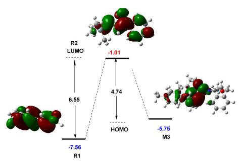
Calculated frontier molecular orbitals of R1, R2, and M3 at the M06-2X/6-31G(d,p) level (unit in eV).
