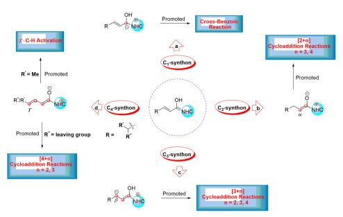
Scheme 2 The formation of different reactive intermediates from the Breslow intermediate
