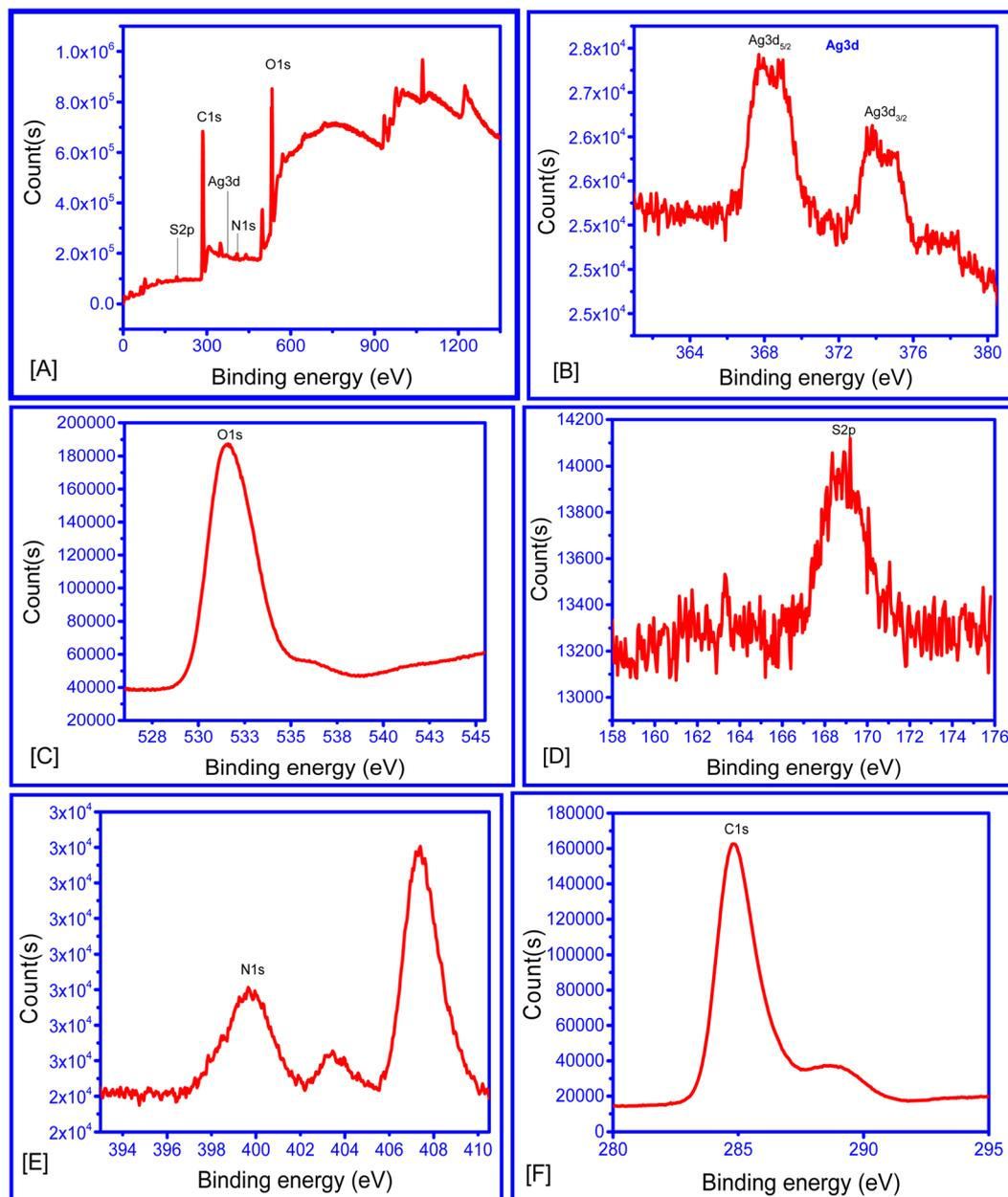
Fig. 5 (A) XPS survey scan of AC–AgNPs, (B) XPS Ag 3d scan, (C) XPS (O 1s scan), (D) XPS S 2p scan, (E) XPS N 1s scan, (F) XPS C 1s scan.
