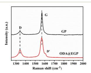
Fig. 3 Raman spectra of GP and ODA@EGP.
