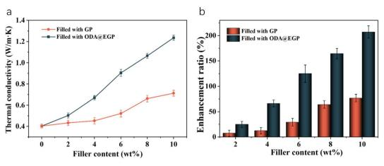
Fig. 7 (a) Thermal conductivity and (b) enhancement ratio of the PE/GP composites with different GP contents
