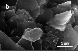
Fig. 1 SEM images of GP platelets: (a) GP and (b) ODA@EGP.
