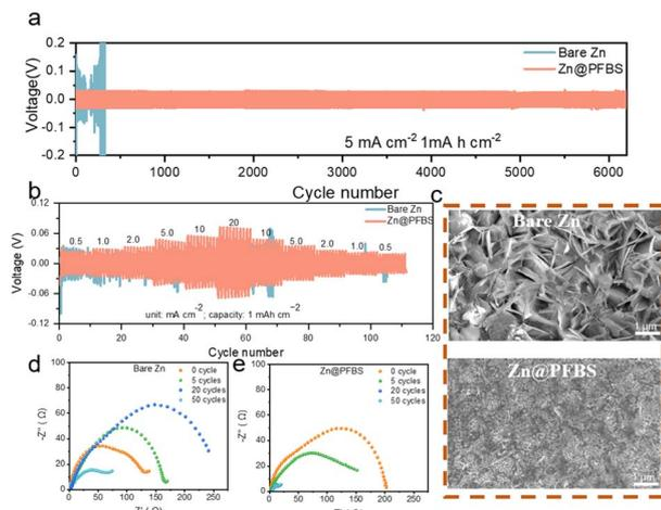
Fig. 5 (a) Long-term cycling performance of symmetric Zn//Zn and Zn@PFBS//Zn@PFBS half-cells at  $5 \text{ mA cm}^{-2}$  to  $1 \text{ mA h cm}^{-2}$ ; (b) rate performance of symmetrical batteries assembled with bare zinc and Zn@PFBS anodes; (c) SEM images of the bare Zn and Zn@PFBS anodes after 100 cycles at  $5 \text{ mA cm}^{-2}$  to  $\text{mA h cm}^{-2}$ ; Nyquist plots of the (d) bare Zn and (e) Zn@PFBS symmetrical batteries at different cycles.
