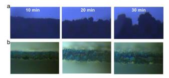
Fig. 2 In situ optical microscopy observations at a current density of 10 mA cm<sup>-2</sup> (a) bare Zn (b) Zn@PFBS.
