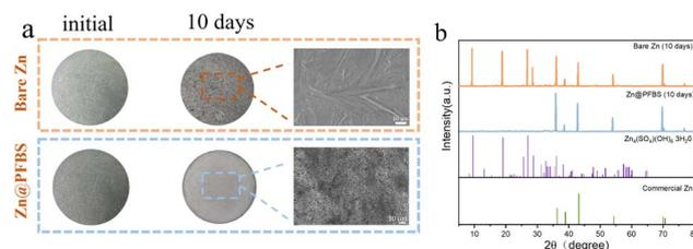
Fig. 4 (a) Optical images and corresponding SEM images of the bare Zn and Zn@PFBS electrodes before and after immersion in a  $2 \text{ M ZnSO}_4$  electrolyte for 10 days; (b) XRD patterns of the bare zinc and Zn@PFBS electrodes after immersion for 10 days.
