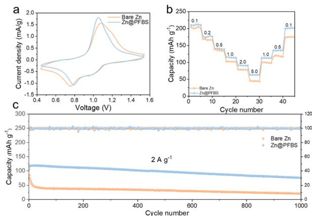
Fig. 6 (a) Cyclic voltammogram of the full cell at a scan rate of  $1 \text{ mV s}^{-1}$ ; (b) rate performance at different current densities; (c) cycle life of Zn@PFBS and bare zinc anodes in a full cell at  $2 \text{ A g}^{-1}$ .
