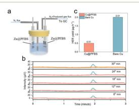
Fig. 3 (a) Schematic diagram and (b) time-voltage curve from in situ EC-GC measurements; (c)  $\rm H_2$  generation rate.
