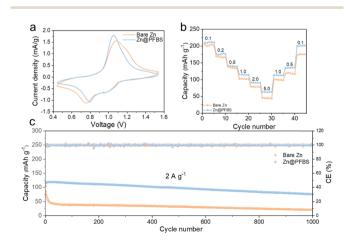
Fig. 6 (a) Cyclic voltammogram of the full cell at a scan rate of 1 mV  $s^{-1}$ ; (b) rate performance at different current densities; (c) cycle life of Zn@PFBS and bare zinc anodes in a full cell at 2 A  $g^{-1}$ .
