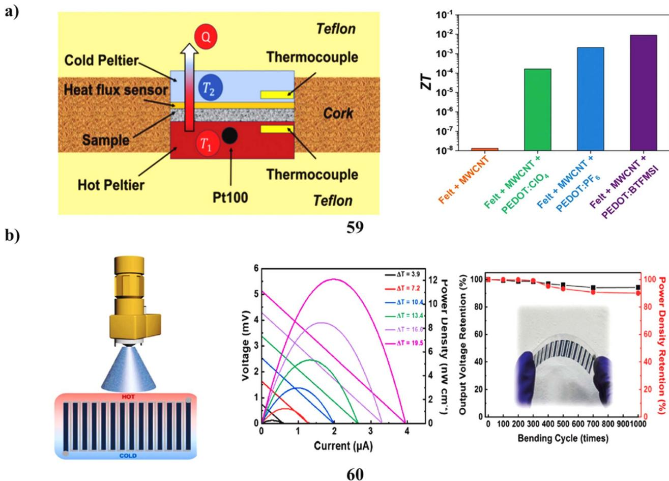
Fig. 32 (a) Electrochemical polymerization based thermoelectric generator (59). (b) Seebeck coefficient study of PEDOT-PSS based high thermoelectric device (60).
