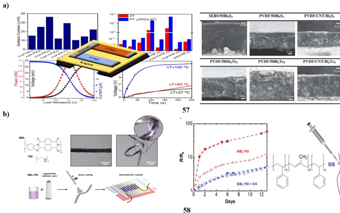
Fig. 31 (a) PVDF/CNT/Bi<sub>2</sub>Te<sub>3</sub> composite based flexible thermoelectric energy (57). (b) Polymer-based n-type yarn for organic TE textiles (58).
