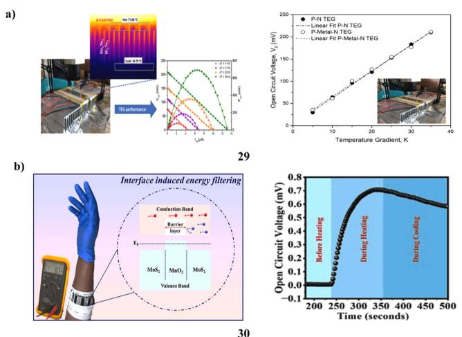
(a) Thermoelectric device study of Bi<sub>2</sub>Te<sub>3</sub>/Sb<sub>2</sub>Te<sub>3</sub> p-n junctions (29). (b) MoS<sub>2</sub>/CF based interface induced energy filtering of TE device (30).
