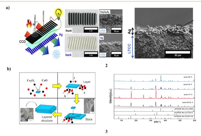
Fig. 2 (a) Spray-coating of ceramic-based thermoelectric generator (2). (b) Thermoelectric study of Ca<sub>7</sub>Co<sub>4</sub>O<sub>9</sub> ceramics (3).
