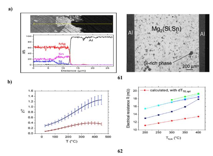
Fig. 33 (a) Seebeck coefficient study of Mg<sub>2</sub>(Si,Sn)-based thermoelectric devices (61). (b) Thermoelectric characteristics of the thermoelectric generator based on Mg<sub>2</sub>(Si,Sn) (62).
