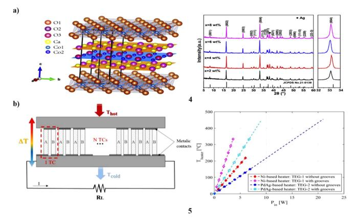
Fig. 3 (a) Liquid-phase sintering study of  $Ca_3Co_4O_9$ -Bi<sub>2</sub>O<sub>3</sub> based ceramics (4). (b) LTCC technology of Ag/PdAg-based ceramic-based thermoelectric generator (5).
