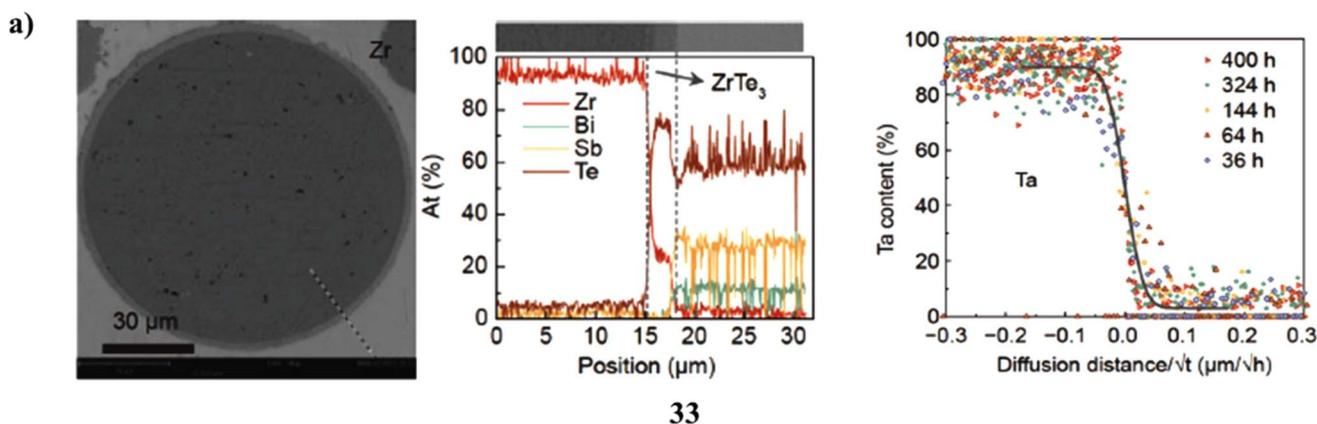
Fig. 18 (a) Metal diffusion barrier screening for thermoelectric Bi<sub>0.5</sub>Sb<sub>1.5</sub>Te<sub>3</sub> (33). (b) Thermoelectric properties of metal chloride complexes (34).
