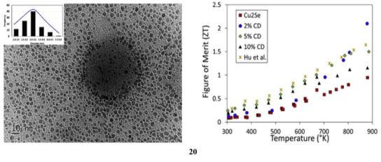
Fig. 11 Gel-like carbon dots based thermoelectric performance of Cu<sub>2</sub>Se (20).
