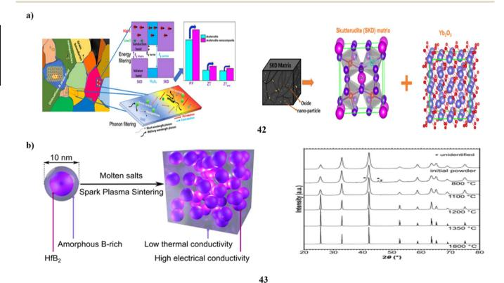
Fig. 23 (a) Skutterudite- $Yb_2O_3$  nanocomposites based thermoelectric device (42). (b) Transport properties of nanoparticle-based boron-rich composites (43).
