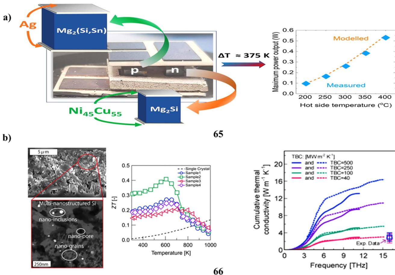
Fig. 35 (a) Thermoelectric study of Mg<sub>2</sub>(Si,Sn)-based thermoelectric generators (65). (b) Multi-nanostructured silicon based thermoelectrics (66).
