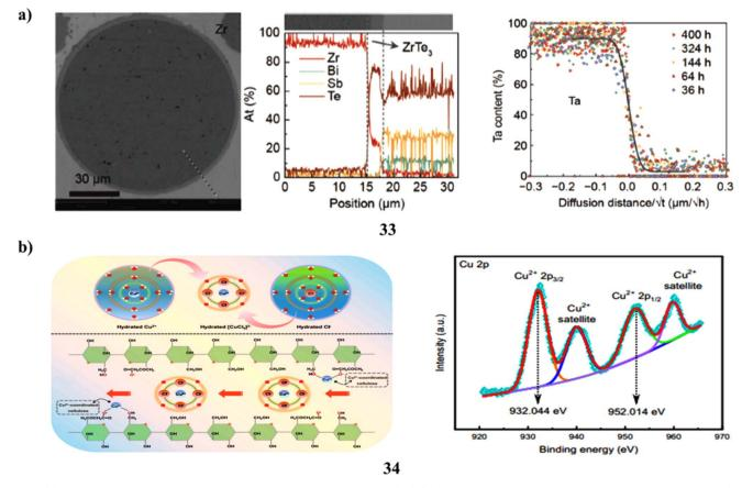
$\textbf{Fig. 18} \quad \textbf{(a) Metal diffusion barrier screening for thermoelectric } \textbf{Bi}_{0.5} \textbf{Sb}_{1.5} \textbf{Te}_{3} \textbf{ (33)}. \textbf{ (b) Thermoelectric properties of metal chloride complexes (34)}.$
