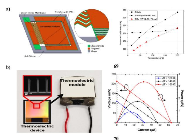
(a) SiGe nanowires-based thermoelectric microgenerators (69). (b) Thermoelectric properties of Si-NWs (70)
