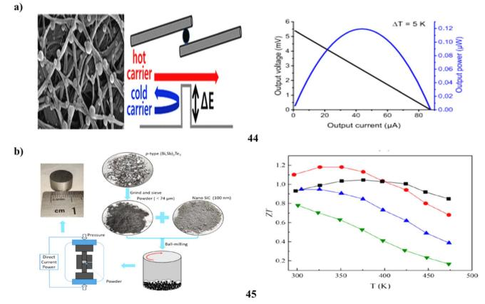
(a) CNP-CNT heterostructures based Thermoelectric device (44). (b) (Bi,Sb)<sub>2</sub>Te<sub>3</sub>-based thermoelectric nano-composites (45).
