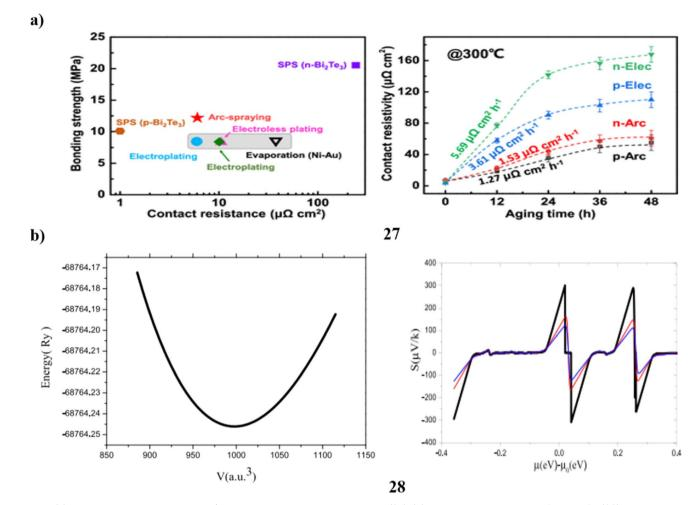
Fig. 15 (a) Thermal tolerance study of Ni/Bi Te based thermoelectric devices (27). (b) Thermoelectric study of Sr<sub>2</sub>EuReO<sub>6</sub> (28).
