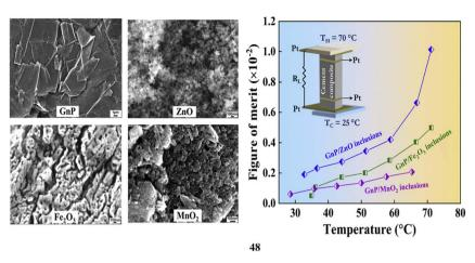
Fig. 26 Thermoelectric figure of merit study of graphene-based metal oxide nanoparticles (48).
