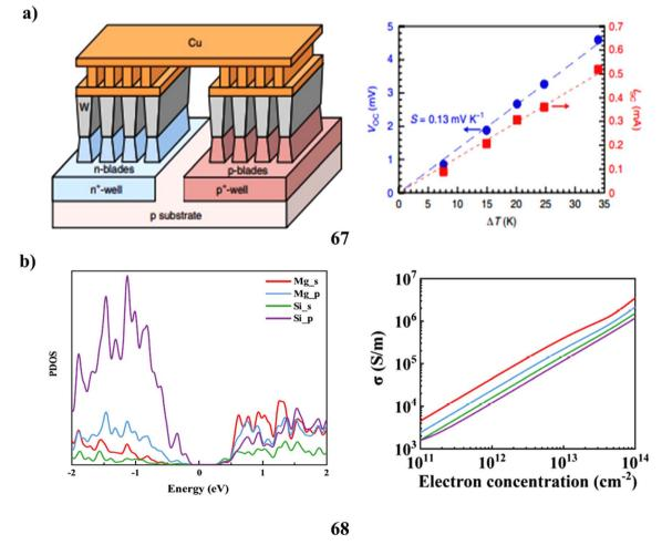
Fig. 36 (a) Silicon CMOS-based thermoelectric generators (67). (b) Mg-Si monolayer-based thermoelectric device (68).
