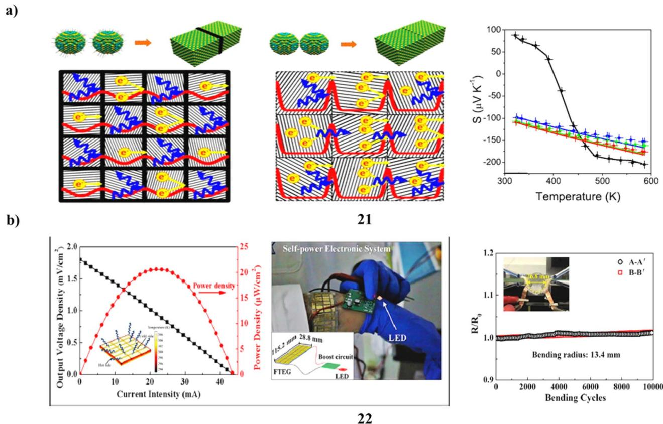
Fig. 12 (a) PbSe nanomaterials-based TE generator (21). (b) Mg<sub>3</sub>Bi<sub>2</sub>-based thermoelectric generator (22).
