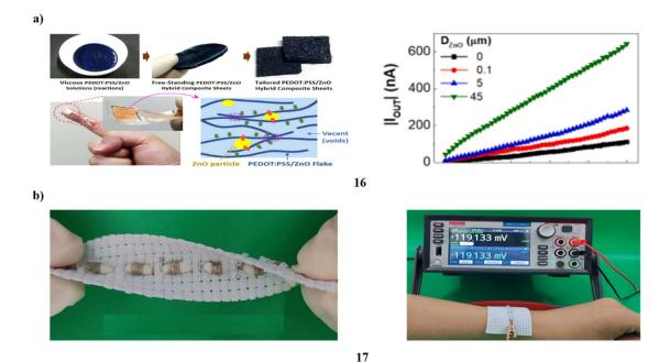
Fig. 9 (a) PEDOT:PSS/ZnO hybrid composites for organic thermoelectric devices (16). (b) Low-grade human body heat gathering device based on ionogel fiber (17).
