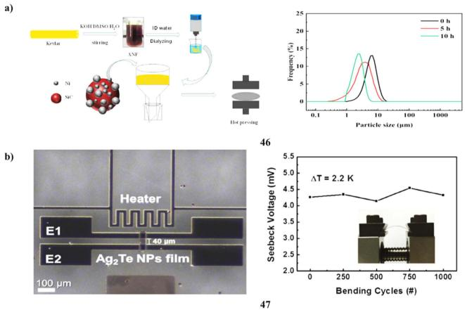
Fig. 25 (a) SiC-nickel nanoparticle-based thermal conductive applications (46). (b) Thermoelectric characteristics of  $\gamma$ -Ag<sub>2</sub>Te nanoparticle (47).
