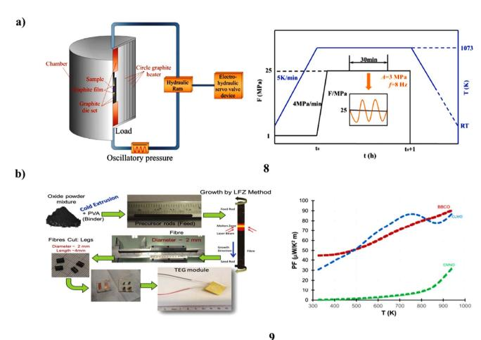
(a) Thermoelectric study of  $Ca_7Co_4O_9$  based ceramics (8). (b) Ceramic legs-based thermoelectric modules (9)
