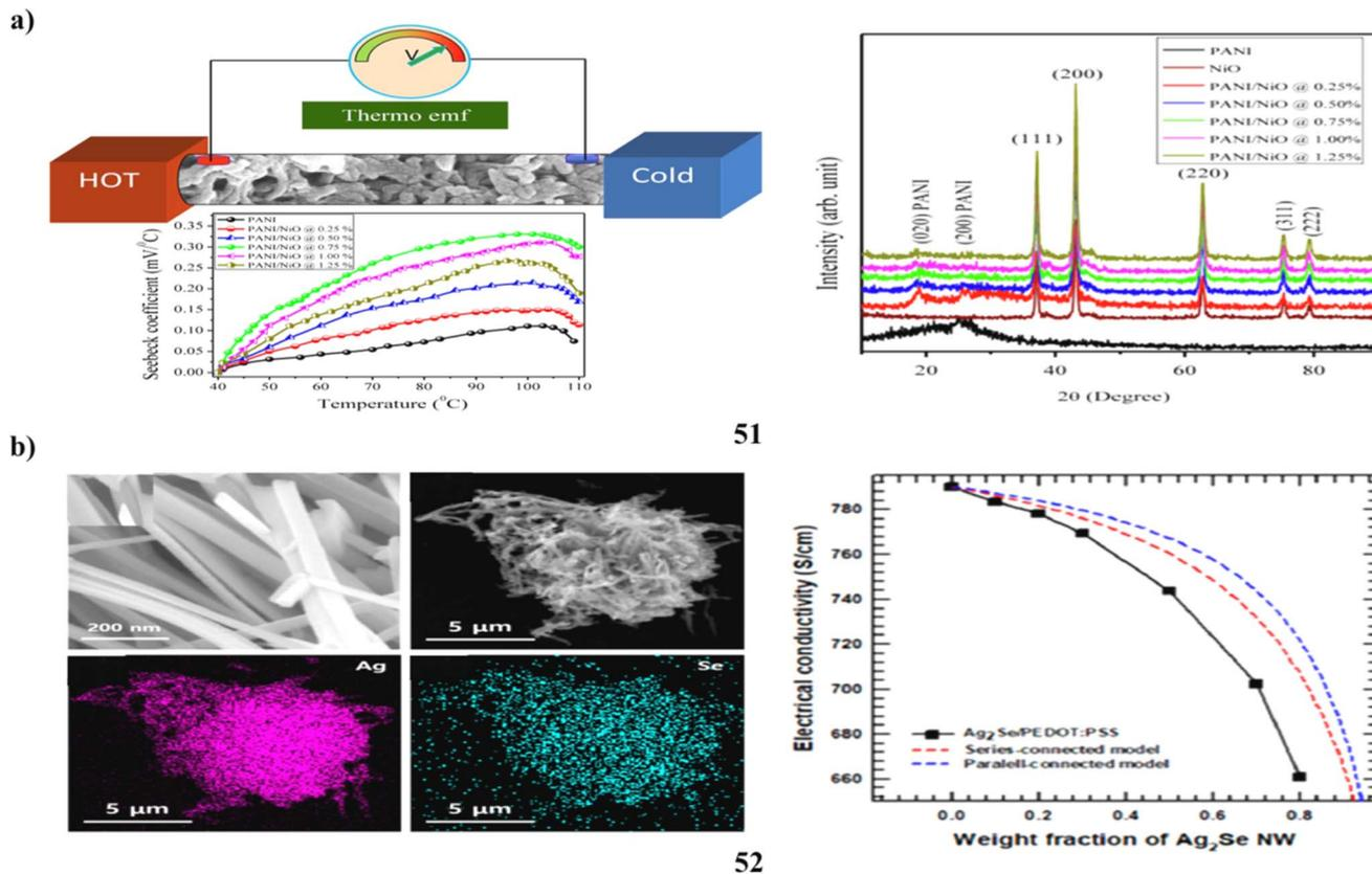
Fig. 28 (a) Polyaniline/nickel oxide-based thermoelectric generator (51). (b) PEDOT:PSS/Ag<sub>2</sub>Se nanowires based thermoelectric applications (52).
