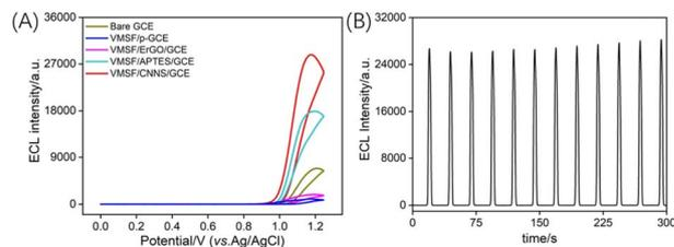
Fig. 4 (A) The  $I_{\text{ECL}}$ -potential obtained on different electrodes in  $10 \mu\text{M}$   $\text{Ru}(\text{bpy})_3^{2+}$  and  $15 \text{ mM}$   $\text{Et}_3\text{N}$ . (B)  $I_{\text{ECL}}$ -time curve obtained on VMSF/CNNS/GCE.
