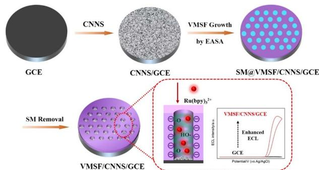
Fig. 1 Illustration for the preparation of VMSF/CNNS/GCE and the improved ECL signals through electrostatic attraction of  $\text{Ru}(\text{bpy})_3^{2+}$  through VMSF nanochannels.
