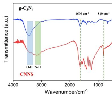
Fig. 2 FTIR spectra of bulk  $\text{g-C}_3\text{N}_4$  and CNNS.
