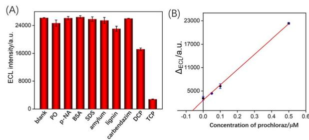
Fig. 7 (A) ECL signal of  $Ru(bpy)_3^{2+}/Et_3N$  system measured on VMSF/CNNS/GCE sensor in presence of single substance or all substances simultaneously. (B) Linear relationship between ECL signal and TCP concentration in orange peel extract.
