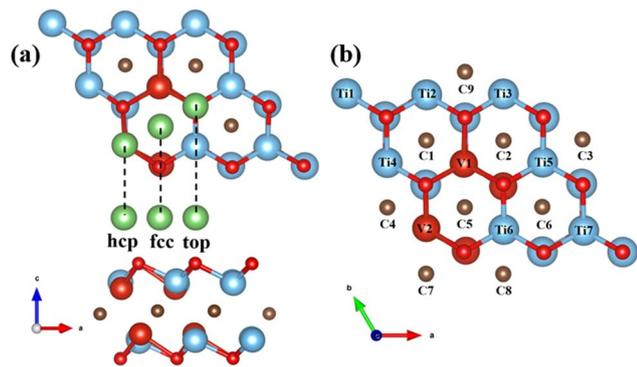
Fig. 3 (a) Top view and side view of three possible lithium-ion adsorption sites on MXene. (b) possible lithium-ion adsorption sites on TiVCO<sub>2</sub>.
