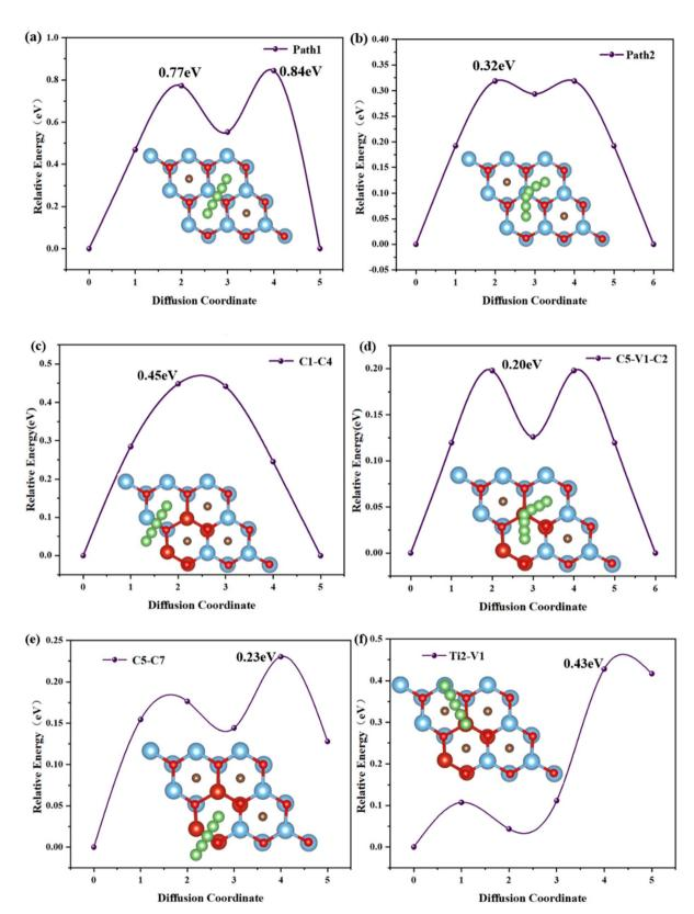
Fig. 5 Diffusion energy barrier and path of lithium ions on the surface of  $Ti_2CO_2$  (a and b) and  $TiVCO_2$  (c-f) monolayers.
