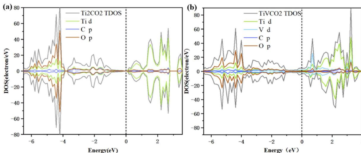
Fig. 2 Total density of states (DOS) and partial density of states (PDOS) of (a) Ti<sub>2</sub>CO<sub>2</sub> and (b) TiVCO<sub>2</sub>. The Fermi level was set to 0 eV.
