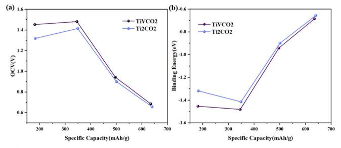
Fig. 7 (a) Change curve of open circuit voltage with specific capacity of  $Ti_2CO_2$  and  $TiVCO_2$ . (b) The relationship between the binding energy of each Li atom and the specific capacity of MXene.
