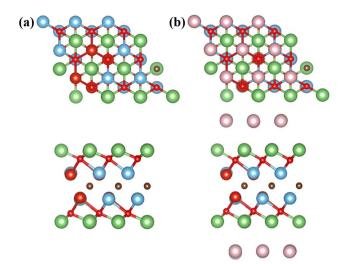
**Fig. 6** Top view and side view of optimized MXene, (a) single layer Li and (b) double layer Li on both sides. The green and pink balls represent the first and second layers of lithium atoms respectively.
