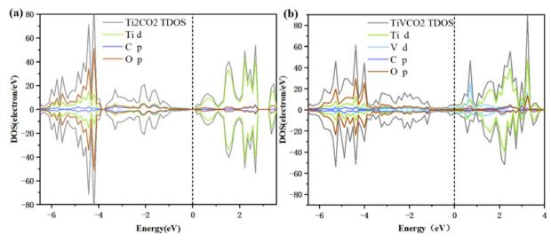
Fig. 2 Total density of states (DOS) and partial density of states (PDOS) of (a) Ti<sub>2</sub>CO<sub>2</sub> and (b) TiVCO<sub>2</sub>. The Fermi level was set to 0 eV.
