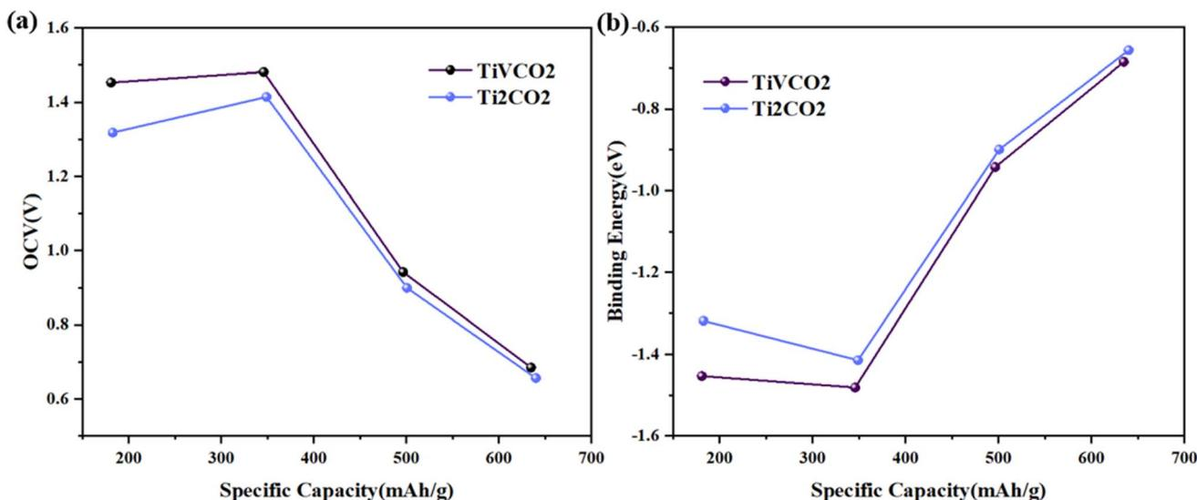
Fig. 7 (a) Change curve of open circuit voltage with specific capacity of  $\text{Ti}_2\text{CO}_2$  and  $\text{TiVCO}_2$ . (b) The relationship between the binding energy of each Li atom and the specific capacity of MXene.
