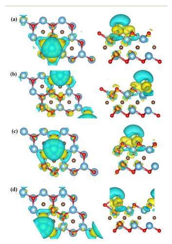
Fig. 4 Differential charge diagrams of Li atoms adsorbed on (a) C5, (b) Ti3, (c) V1, (d) V2 respectively.
