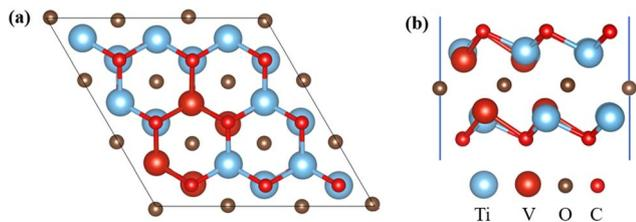
Fig. 1 Geometric model of TiVCO<sub>2</sub>. Top (a) and side (b) view.
