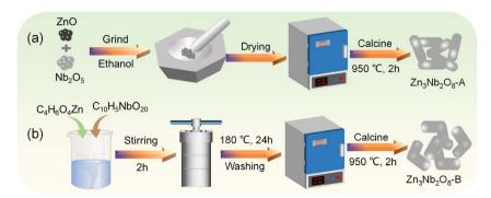
Fig. 1 Schematic illustration of Zn<sub>3</sub>Nb<sub>2</sub>O<sub>8</sub> materials synthesized by (a) solid-state reaction and (b) solvothermal reaction.
