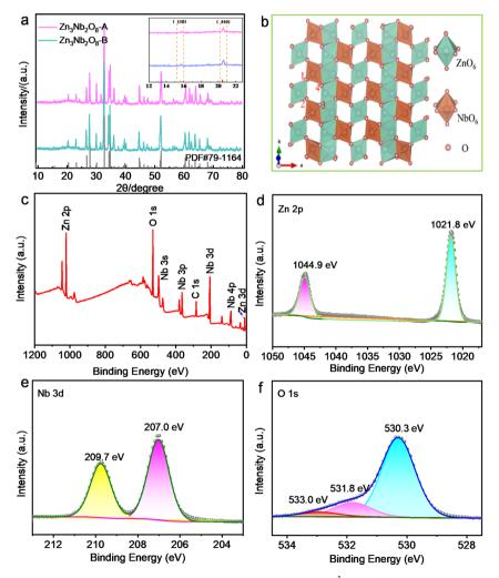
Fig. 2 (a) XRD pattern of  $Zn_3Nb_2O_8$ -A and  $Zn_3Nb_2O_8$ -B calcined at 950 °C at 10 °C min<sup>-1</sup> in air. (b) Crystal structure of  $Zn_3Nb_2O_8$ , (c) XPS survey spectra of  $Zn_3Nb_2O_8$ -B; XPS spectra of  $Zn_3Nb_2O_8$ -B for (d)  $Zn_3Nb_2O_8$ -B f
