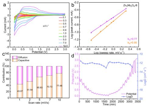
Fig. 5 (a) CV curves of  $Zn_3Nb_2O_8$ -B from 0.1 to 10.0 mV s<sup>-1</sup>; (b) plots of log(i) vs. log(v) of the  $Zn_3Nb_2O_8$ -B/Li cell; (c) contribution ratios of diffusion- and capacitive-controlled capacities at different scan rates. (d) GITT curves of  $Zn_3Nb_2O_8$ -B at 0.01–3.00 V.
