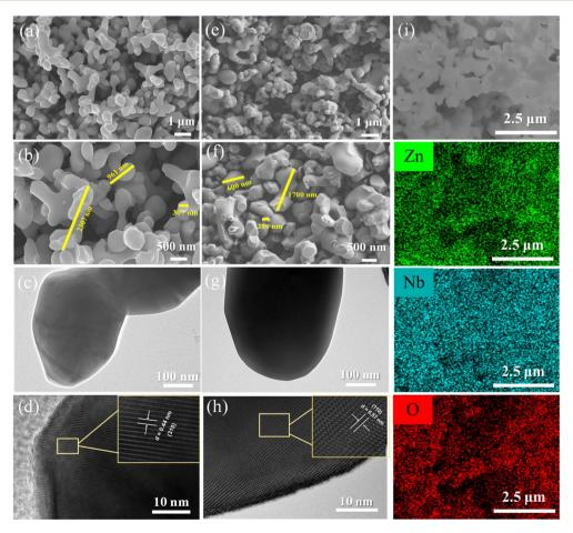
Fig. 3 (a and b) SEM images, (c) TEM image and (d) HRTEM image of  $Zn_3Nb_2O_8$ -A; (e and f) SEM images, (g) TEM image, (h) HRTEM image and (i) EDS mapping images of  $Zn_3Nb_2O_8$ -B.
