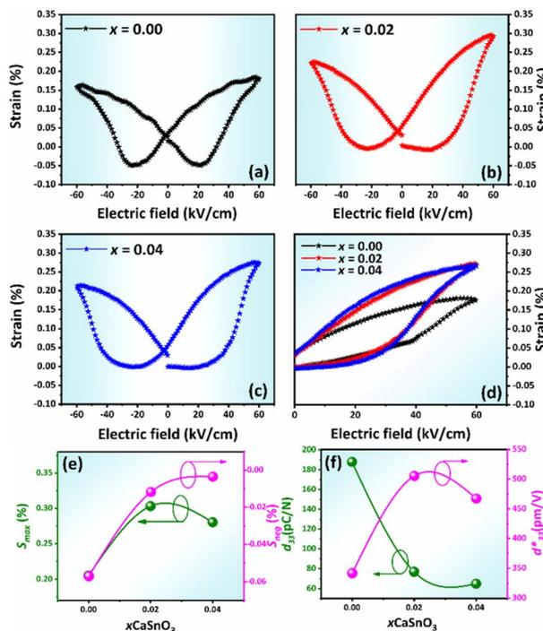
Fig. 7 Electro-strain and piezoelectric properties of the samples at different CSO content and RT: (a–c) bipolar  $S$ - $E$  loop versus CSO content for the  $x = 0.00$ – $0.04$  samples, (d) unipolar  $S$ - $E$  loop versus CSO content, (e)  $S_{\text{max}}$  and  $S_{\text{neg}}$  versus CSO content, and (f)  $d_{33}$  and  $d_{33}^*$  value as a function of CSO content.
