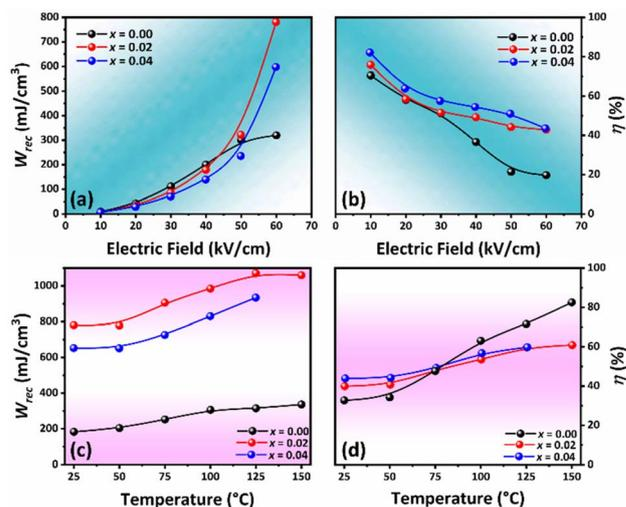
Fig. 6 Energy storage properties of the samples: (a)  $W_{\text{rec}}$  vs. electric field, (b)  $\eta$  vs. applied electric field, (c)  $W_{\text{rec}}$  vs. temperature, and (d)  $\eta$  vs. temperature.
