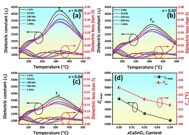
Fig. 4 (a)–(c) Temperature dependence of dielectric constant ( $\epsilon_r$ ) and dielectric loss ( $\tan \delta$ ) of the ceramics as a function of CSO content and (d) plots of  $\epsilon_{r,\text{max}}$  and  $T_m$  as a function of CSO content.
