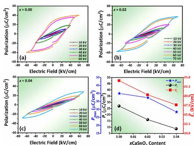
Fig. 5 Polarization–electric field ( $P$ – $E$ ) hysteresis loops of  $(1 - x)$  [0.99BNKT–0.01BMN]– $x$ CSO ceramics at RT and different electric fields: (a)  $x = 0.00$ , (b)  $x = 0.02$ , (c)  $x = 0.04$ , and (d) plots of  $P_{\text{max}}$ ,  $P_r$ , and  $E_c$  as a function of CSO content.
