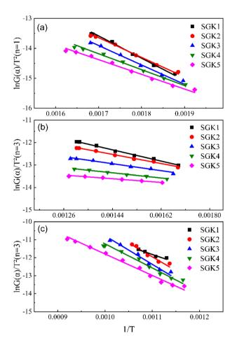
Fig. 6 Linear regression curves with  $K_2CO_3$  (a) the first-stage (<350 °C); (b) the second-stage (350–650 °C); (c) the third-stage.
