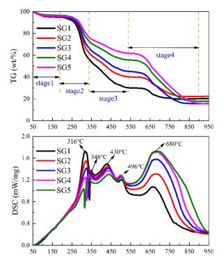
Fig. 1 TG-DSC curves of the blends without K<sub>2</sub>CO<sub>3</sub>.
