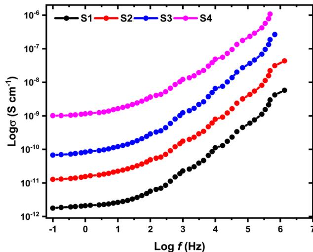
Fig. 8 The relationship between  $\log \sigma$  and  $\log f$  for both HPMC/PEDOT:PSS composite films and HPMC/PEDOT:PSS films incorporating SnO<sub>2</sub> nanoparticles.
