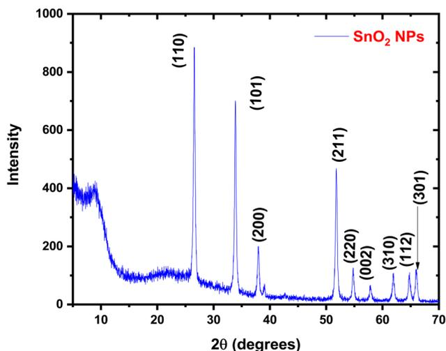
Fig. 1 XRD pattern of pure SnO<sub>2</sub> nanoparticles.
