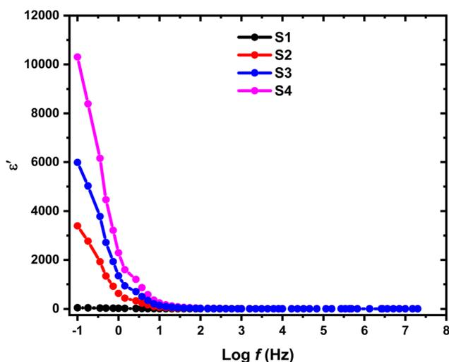
Fig. 9 Variation in dielectric constant ( $\epsilon'$ ) with  $\log(f)$  for HPMC/PEDOT:PSS composite and HPMC/PEDOT:PSS loaded with SnO<sub>2</sub> NPs.
