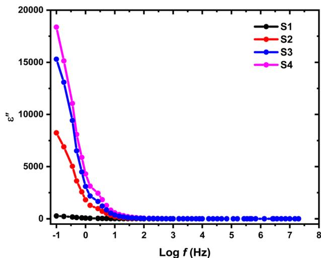
Fig. 10 Variation in dielectric loss ( $\epsilon''$ ) with  $\log(f)$  for HPMC/PEDOT:PSS composite and HPMC/PEDOT:PSS loaded with SnO<sub>2</sub> NPs.
