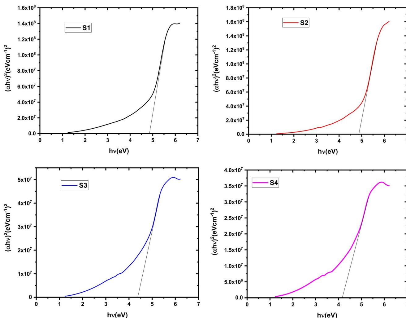
Fig. 6 Tauc plot for determining the direct band gap ( $E_{dg}$ ) of HPMC/PEDOT:PSS composites with varying SnO<sub>2</sub> nanoparticle loadings.
