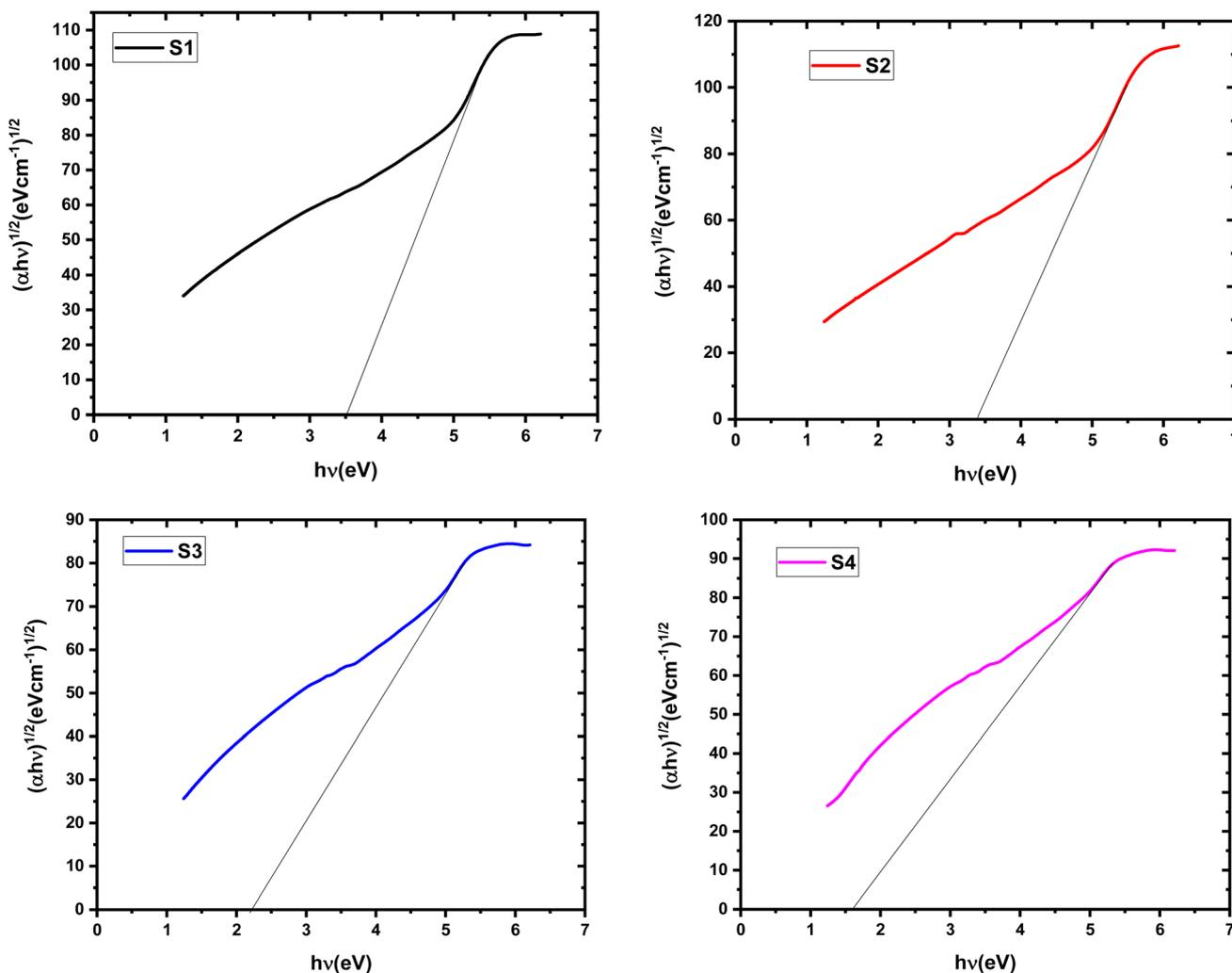
Fig. 7 Tauc plot for determining the indirect band gap ( $E_{ig}$ ) of HPMC/PEDOT:PSS composites with varying SnO<sub>2</sub> nanoparticle loadings.
