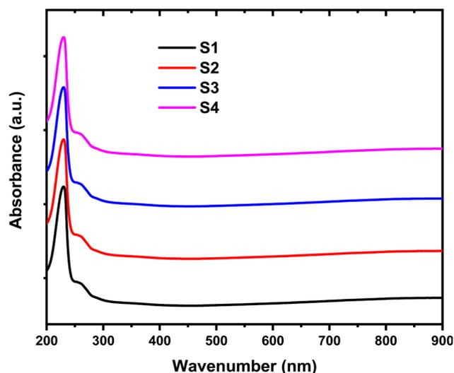
Fig. 5 UV-Vis absorption spectra of the HPMC/PEDOT:PSS composite and HPMC/PEDOT:PSS nanocomposites containing different SnO<sub>2</sub> nanoparticle loadings.
