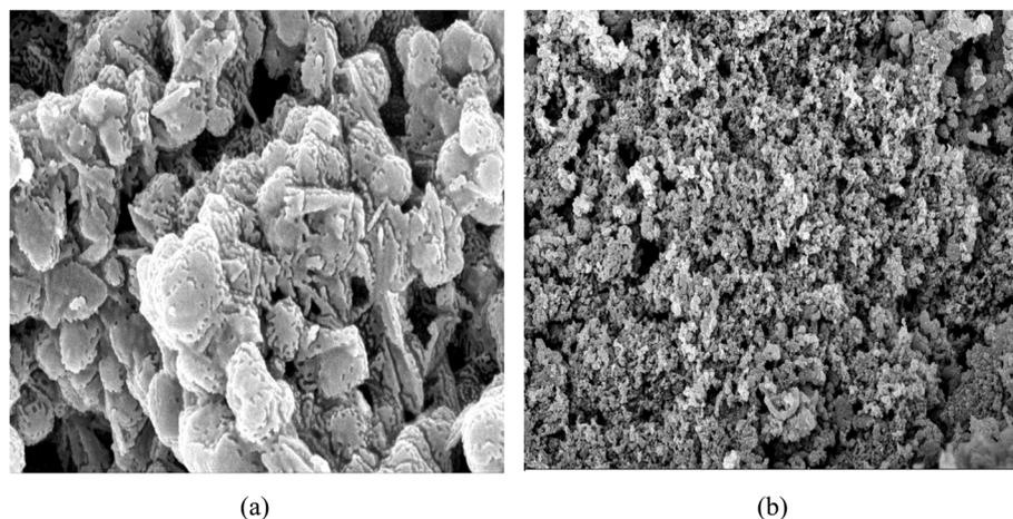
Fig. 4 FESEM images (a) HPMC/PEDOT:PSS, (b) HPMC/PEDOT:PSS/0.007 g SnO<sub>2</sub> nanocomposite.
