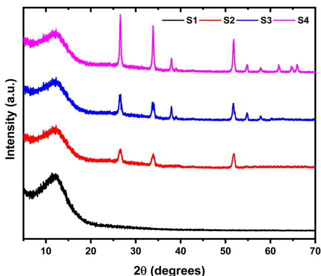
Fig. 2 XRD pattern of HPMC/PEDOT:PSS ternary blend and HPMC/PEDOT:PSS doped with SnO<sub>2</sub> nanoparticles.
