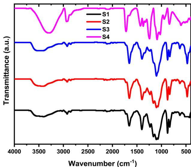
Fig. 3 FT-IR spectra of HPMC/PEDOT:PSS ternary blend doped with SnO<sub>2</sub> nanoparticles.
