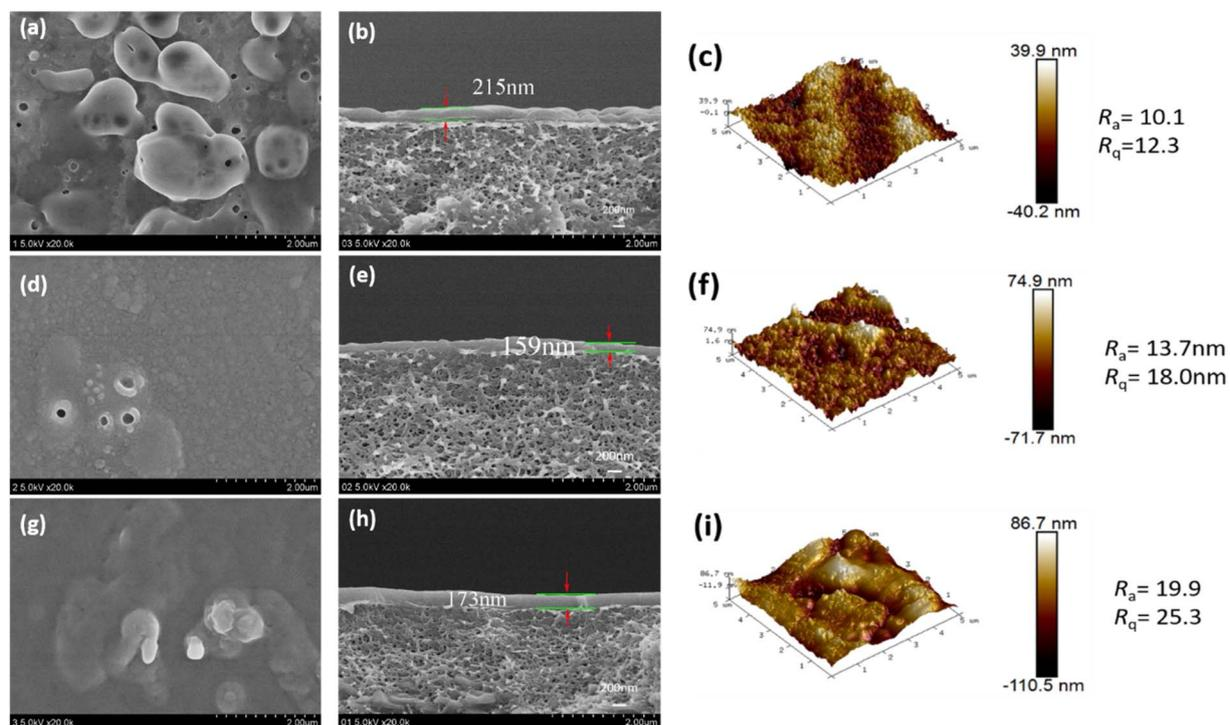
Fig. 5 SEM images of CPVC composite LNF membrane at different GA : PEI ratio: (a and b) 1 : 3, (d and e) 2.5 : 7.5, and (g and h) 3 : 9; and AFM images of LNF membrane at different ratio of GA : PEI; (c) 1 : 3, (f) 2.5 : 7.5, and (i) 3 : 9.
