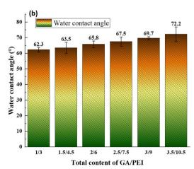
Fig. 6 Effect of water contact angle on CPVC composite LNF membrane; (a) effects of the total content of TA/PEI ratio on hydrophilicity of membrane surface; (b) effects of the total content of GA/PEI on hydrophilicity of membrane surface.
