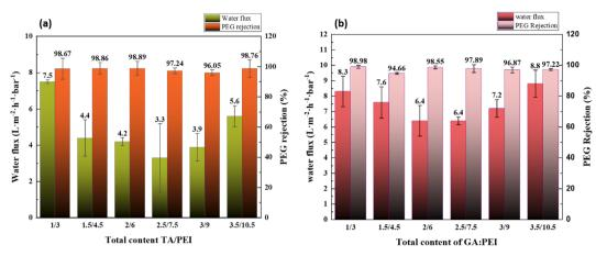
Fig. 7 (a) Effects of total content of TA: PEI ratio on the pure water flux and PEG800 retention rate on CPVC composite LNF membrane; (b) effects of total content of GA: PEI ratio on the pure water flux and PEG800 retention rate on CPVC composite LNF membrane.
