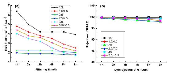
Fig. 9 Stability of CPVC composite LNF membrane in treating simulated RB5 dye wastewater for TA/PEI. (a) Filtration time per hour of RB5 wastewater for TA/PEI; (b) rejection rate of RB5 dye wastewater per hour for TA/PEI.
