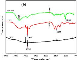
Fig. 3 (a) ATR-FTIR spectra of TA: PEI CPVC composite loose nanofiltration membrane; (b) ATR-FTIR spectra of GA: PEI CPVC composite loose nanofiltration membrane.
