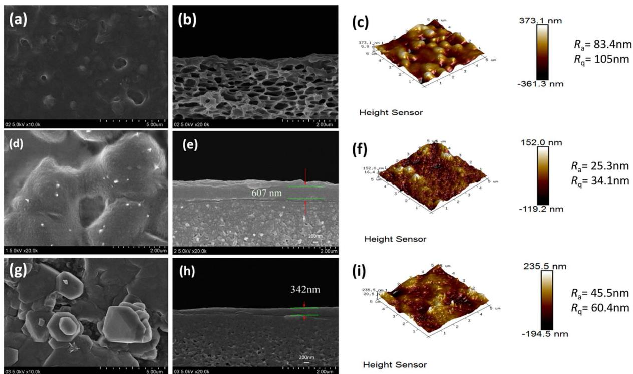
Fig. 4 SEM images of CPVC composite LNF membrane at different TA : PEI ratio: (a and b) 1 : 3, (d and e) 2.5 : 7.5, and (g and h) 3 : 9; and AFM images of LNF membrane at different ratio of TA : PEI; (c) 1 : 3, (f) 2.5 : 7.5, and (i) 3 : 9.
