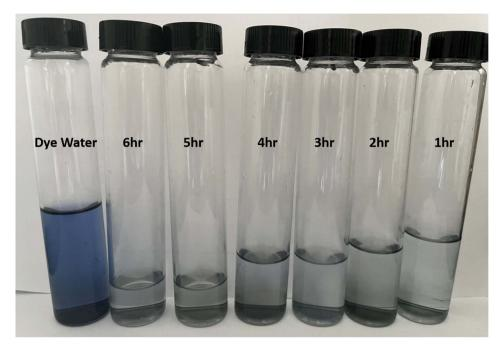
Fig. 2 Filtration of dye wastewater for six hours.
