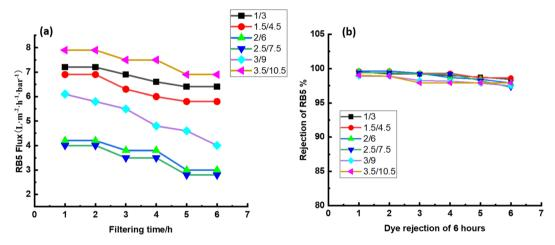
Fig. 10 Stability of CPVC composite LNF membrane in treating simulated RB5 dye wastewater for GA/PEI. (a) Filtration time per hour of RB5 wastewater for GA/PEI; (b) rejection rate of RB5 dye wastewater per hour for GA/PEI.
