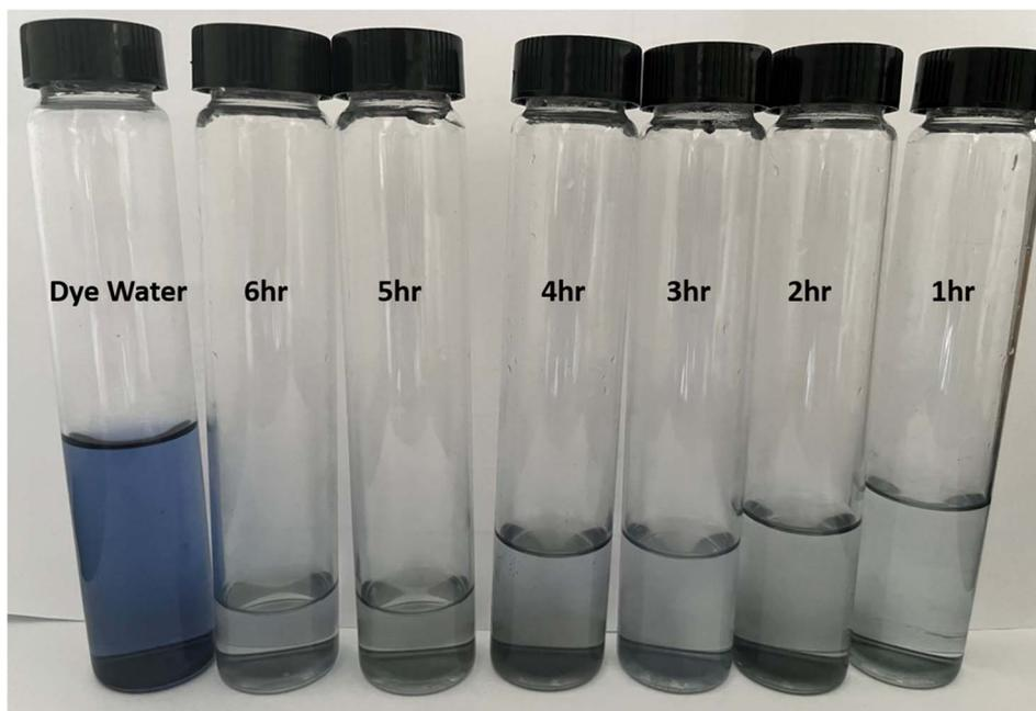
Fig. 2 Filtration of dye wastewater for six hours.
