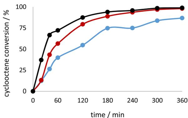
Fig. 7 Kinetic profile for cyclooctene conversion when using TBHP in water as oxidant with the catalysts  $3\text{H}\cdot 2\text{CH}_3\text{CN}$  (red),  $3\text{H}^{\text{w}}$  (blue) and  $3\text{H}$  (black).
