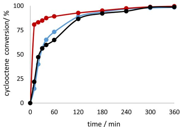
Fig. 6 Kinetic profile for cyclooctene conversion when using TBHP in decane as oxidant with the catalysts  $3\text{H}\cdot 2\text{CH}_3\text{CN}$  (red),  $3\text{H}^{\text{w}}$  (blue) and  $3\text{H}$  (black).
