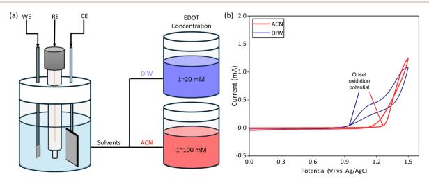
Fig. 1 Electrodeposition diagram. (a) Experimental design. WE, RE, and CE represent working electrode, reference electrode, and counter electrode, respectively. DIW and ACN represent deionized water and acetonitrile. (b) An example to obtain the onset oxidation potential for 20 mM EDOT in the DIW and ACN according to the cyclic voltammograms.
