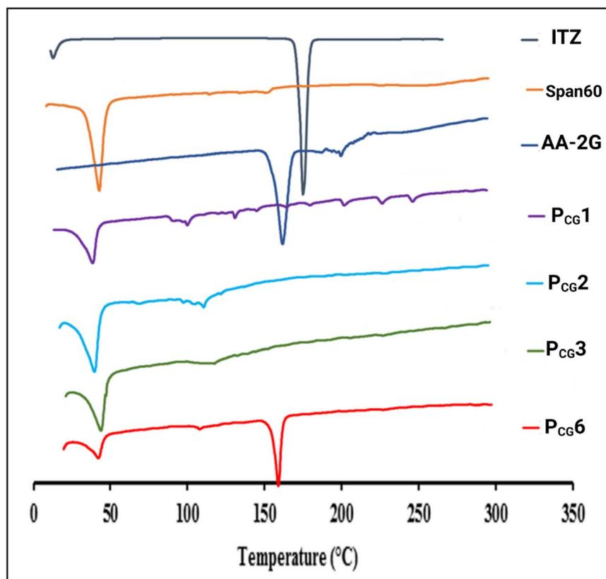
Fig. 3 Differential scanning calorimetry (DSC) thermograms of ITZ, Span 60, ascorbyl glucoside AA-2G, P<sub>CG1</sub>, P<sub>CG2</sub>, P<sub>CG3</sub>, and P<sub>CG6</sub>. P<sub>CG1</sub>: plain glucospanlastics containing 10 mg AA-2G. P<sub>CG2</sub>: ITZ-glucospanlastics containing 10 mg AA-2G and 10 mg ITZ. P<sub>CG3</sub>: ITZ-glucospanlastics containing 10 mg AA-2G and 20 mg ITZ. P<sub>CG6</sub>: ITZ-glucospanlastics containing 20 mg AA-2G and 20 mg ITZ.
