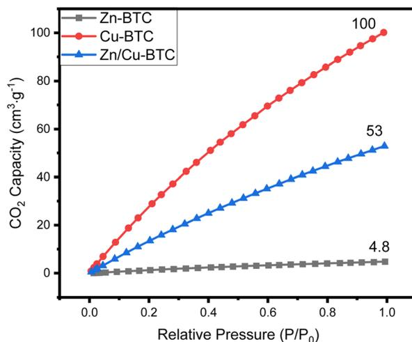
Fig. 5 The CO<sub>2</sub> capacity of Zn/Cu-BTC, Cu-BTC and Zn-BTC at 298 K.
