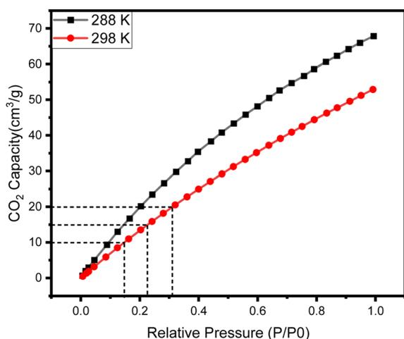
Fig. 7 The  $\text{CO}_2$  adsorption isotherms of Zn/Cu-BTC at 288 K and 298 K.
