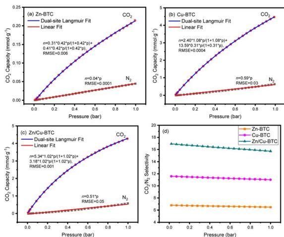
Fig. 6  $\text{CO}_2$  and  $\text{N}_2$  adsorption isotherms of Zn-BTC (a), Cu-BTC (b) and Zn/Cu-BTC (c) at 298 K and the  $\text{CO}_2/\text{N}_2$  selectivity (d) of the three MOFs; the blue curves and red lines in (a)–(c) are the fitting curves.
