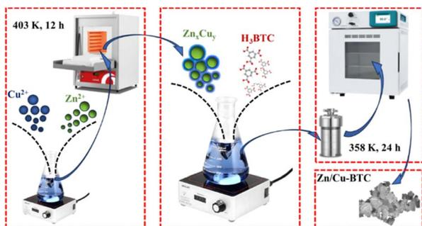
Fig. 1 Synthesis process flowchart of Zn/Cu-BTC.
