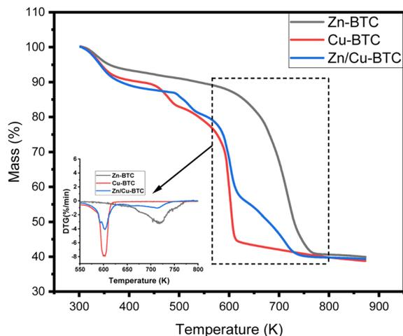
Fig. 4 TGA of Zn-BTC, Cu-BTC and Zn/Cu-BTC samples.
