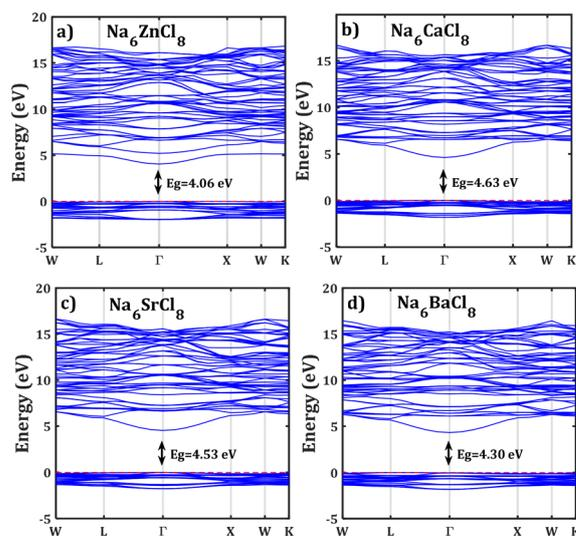
Fig. 2 Band structure of the Na<sub>6</sub>MCl<sub>8</sub> (M = Zn, Ca, Sr, Ba). The computed energy gap ( $E_g$ ) are shown in each case. Horizontal red line represents the Fermi level.
