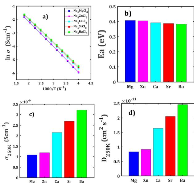
Fig. 4 (a) Arrhenius dependence of Na conductivity ( $\sigma$ ) with the temperature ( $T$ ) of Na<sub>6</sub>MCl<sub>8</sub> structures, (b) their respective activation energy (*E<sub>a</sub>*), (c) conductivity ( $\sigma_{250 K}$ ) and (d) diffusivity (*D*<sub>250 K</sub>) at 250 K.
