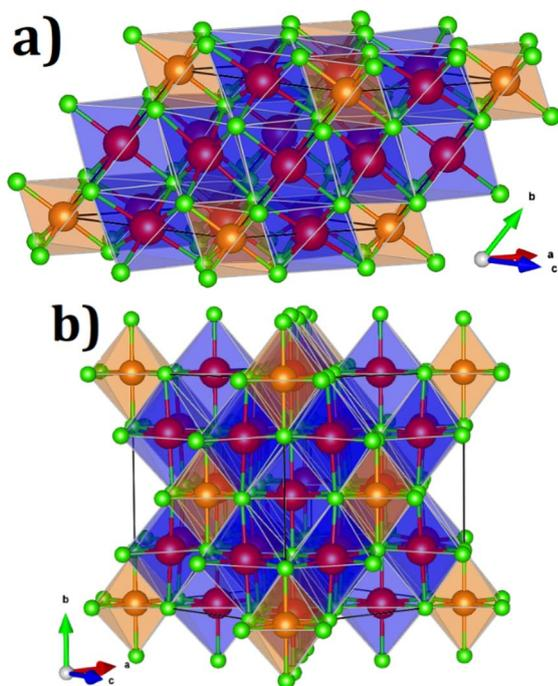
Fig. 1 (a) Primitive and (b) conventional representations of  $\text{Na}_6\text{MCl}_8$  lattice structures (space group  $Fm\bar{3}m$ ). Blue and green balls represent the  $\text{Na}^+$  and  $\text{Cl}^-$  ions and orange and blue polyhedral represent the  $[\text{MCl}_6]$  and  $[\text{NaCl}_6]$  octahedral, respectively.
