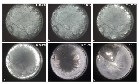
Fig. 2 Representative time-lapse images of the glass transition process upon warming in 49% DMSO. Images taken at chamber-wall temperatures of (a) -135 °C, (b) -130 °C, (c) -125 °C, (d) -120 °C, (e) -115 °C, (f) -110 °C. Source light intensity was adjusted manually in real time to enable consistent measured intensity at the camera (and thereby consistent visual contrast).
