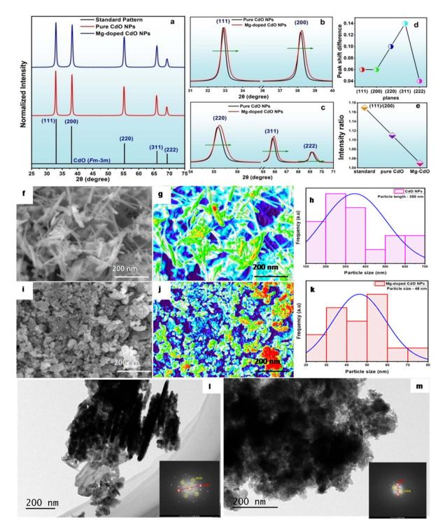
Fig. 2 XRD patterns of pure and Mg-doped CdO NPs, (a) XRD (b and c) zoomed-in portions of the (d) peak shift difference with respect to crystallographic planes (e) normalized peak intensity ratios and FE-SEM images of the (f-h) pure and (i-k) Mg-doped CdO NPs (l and m) HR-TEM Images of the pure and Mg doped CdO NPs (inset: FFT pattern).
