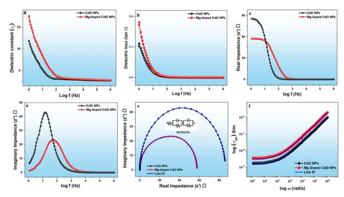
Variation of frequency dependent behaviour of pure and Mq-doped CdO NPs including (a) dielectric constant (b) dielectric loss, (c) z', (d) z'', (e) Nyquist plot and (f) Jonscher's power law.
