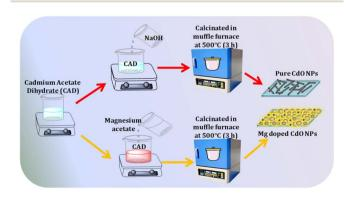
Fig. 1 Schematic of co-precipitation synthesis for pure CdO and Mg-doped CdO NPs.
