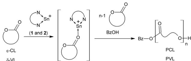
Scheme 2 ROP of  $\delta$ -VL and  $\epsilon$ -CL catalysed by **1** and **2** using BzOH as initiator.
